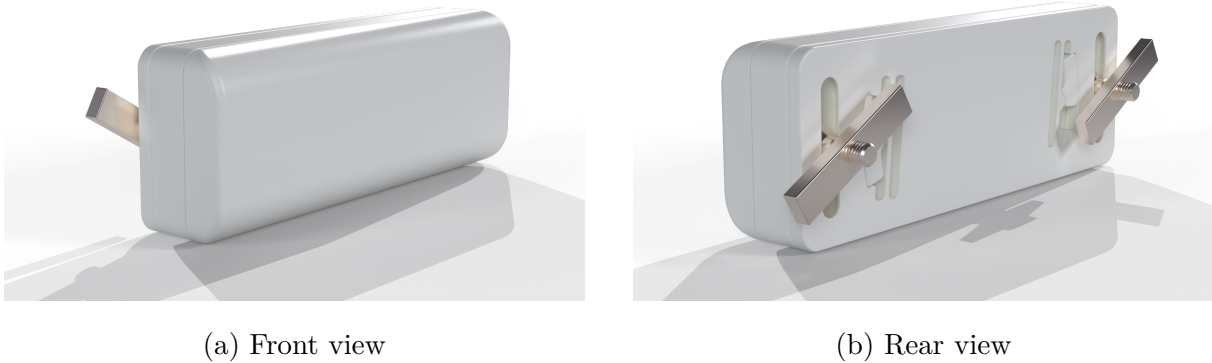
Figure 9.1: Final vibration sensor design shown from front and rear views.
