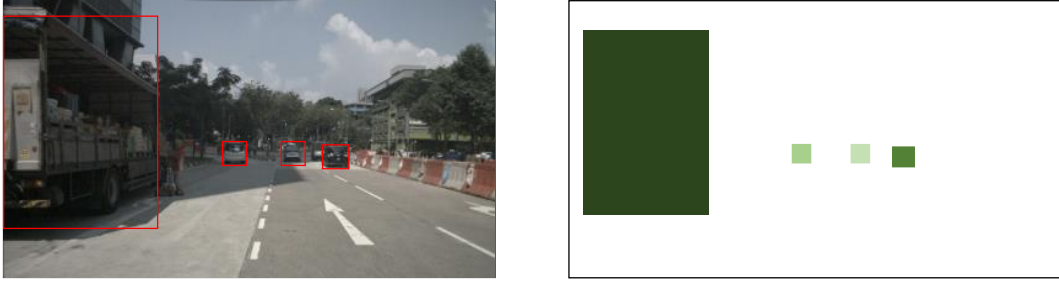
(a) RGB image with 2D-BBs. Source of the picture is the dataset [1]. (b) Camera-radar associated bounding box heatmap \Upsilon representing the depth of the object. Lighter color corresponds to larger depth.
