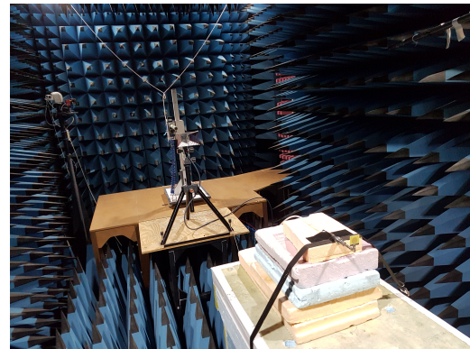
Figure 3.21: Anechoic chamber with the octagonal antenna visible during measurement.
