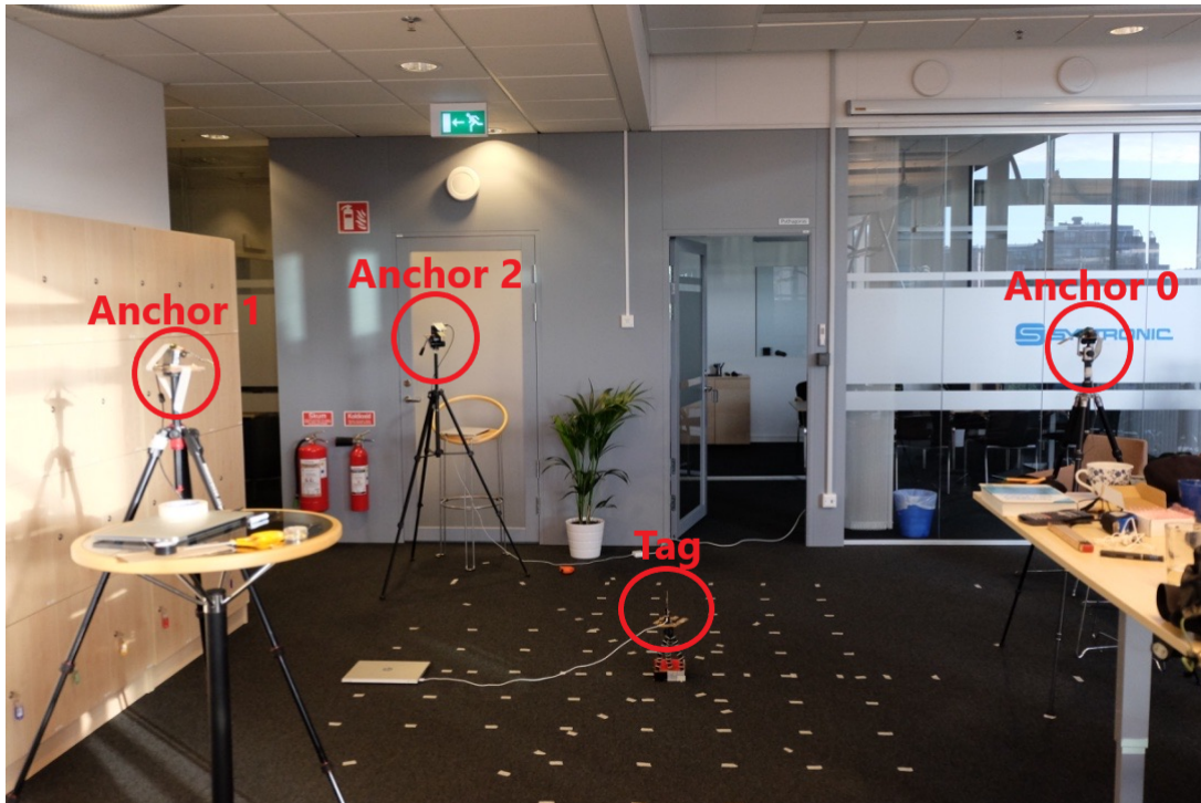
Figure 3.37: Placement of anchors in the LOS setup. White dots on the floor are the chosen locations where the tag will be placed to acquire position estimates. For a more detailed overlook of the positions see figure 3.35 in previous section.
