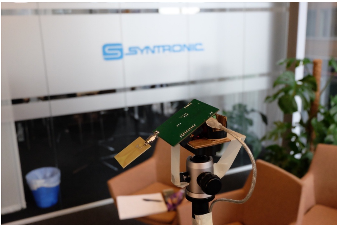
Figure 3.42: Vivaldi antenna directed towards the centre of the measuring area.
