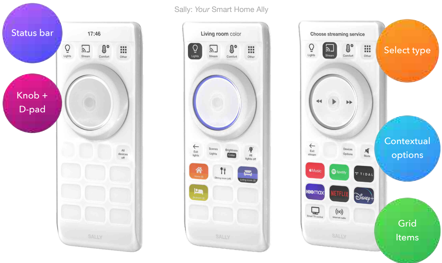
Figure 33. Three different uses of the device. The left image showing how it looks when not in use. The middle showing lights selected. The right one controlling streaming services.
