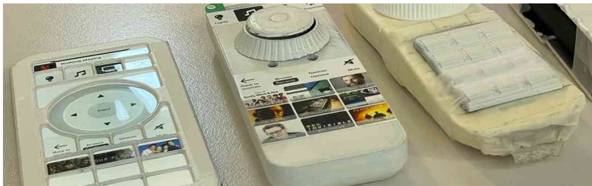
Figure 27. photo of all mockups and prototypes used. Hybrid digital prototype (left), size mockup (middle left), button examples mounted on early mockup (middle right and right).
