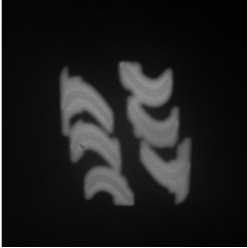
Figure 3.1: Nominal layer image of a single layer showing six turbine blades being simultaneously melted within the electron beam melting (EBM) build chamber. The darker areas correspond to cold powder, while the brighter regions indicate higher temperatures. The melted geometry is surrounded by sintered powder.
