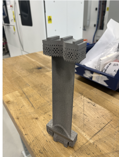
Figure 1.1: A titanium aerospace turbine blade manufactured via Electron Beam Melting.
