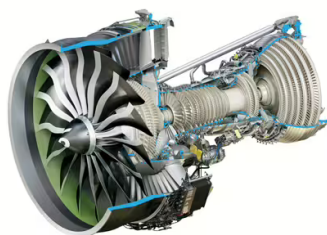
Figure 1.3: The GE9X turbofan engine, developed by GE Aerospace for the Boeing 777X.
