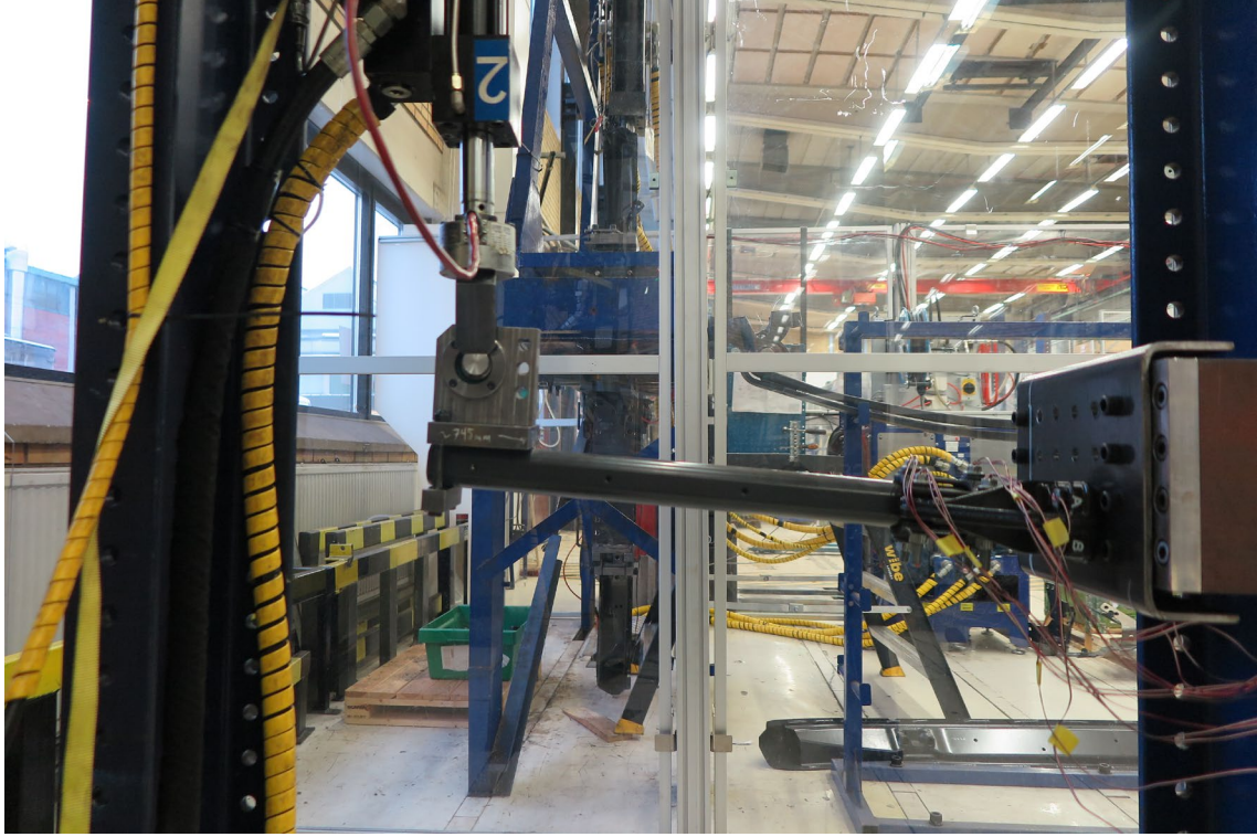
Figure 9: The cylinder to the left applies the load in global x-direction at the end of the beam.
