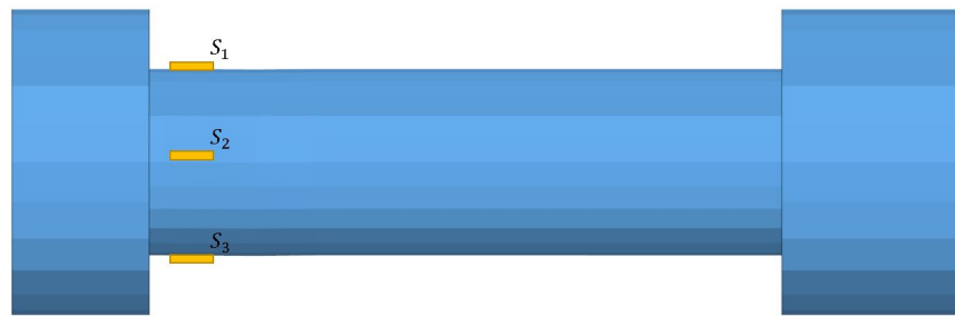
Figure 10: Schematic figure of the strain gauges applied on the bolts to create two half Wheatstone bridges.
