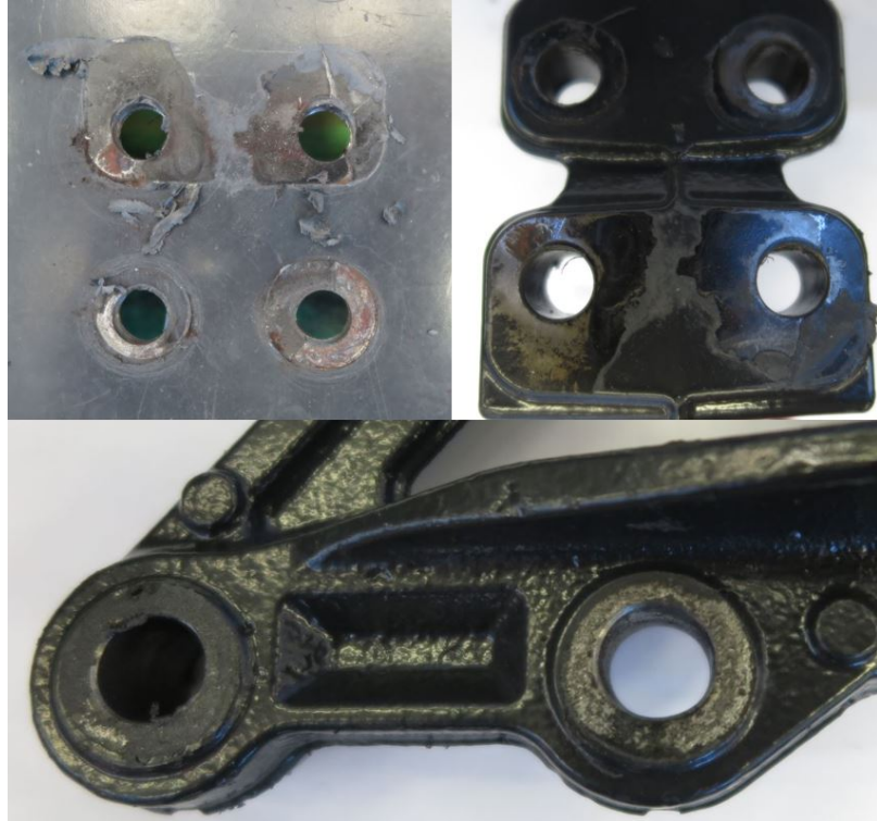
Figure 18: The wear of clamped components. The top figures show the wear of the frame to the left and the back of the frame bracket where the frame bolts are located to the right. The bottom picture shows the wear of the frame bracket, where bolt 5 was located to the right and bolt 6 to the left.
