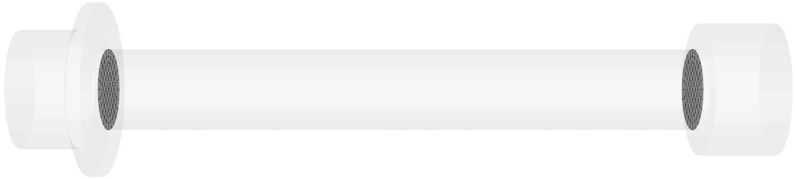
Figure 6: Surface sections where the bending stresses are extracted for the bolt evaluation script. The section where the stresses for the head are evaluated is seen to the left and to the right for the bolt nut.
