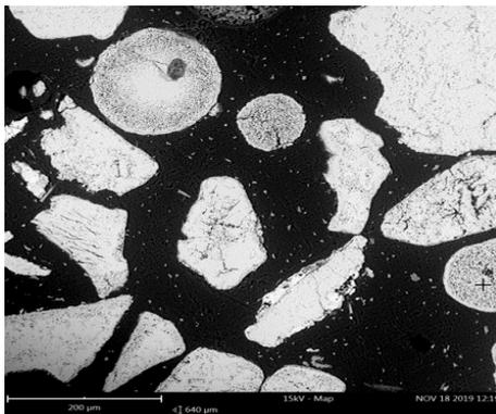
**Figure 3.17:** Cross sectional elemental combined map SEM analysis of the oxygen carrier from the 100 kW unit pilot plant at Chalmers University (color identified)
