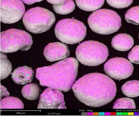
**Figure 3.7:** Surface elemental combined map SEM analysis on the alkali dosed OC (color identified)
