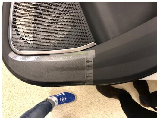
Figure 6.5: *Scratch & wear resistant tape applied to a prototype lower cover.*
