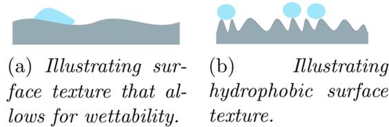
Figure 4.13: *Illustrating two different texture types with regard to liquid adhesion.*
