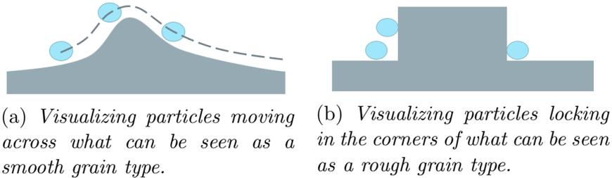
Figure 4.11: *Principle texture type for particle adhesion.*
