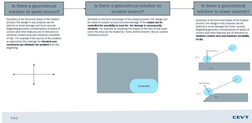
Figure 7.2: Design guideline section Prevention of scratching based on geometry.
