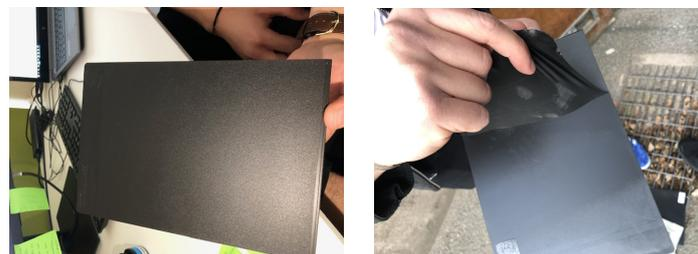
(a) *Spray plastic applied to a test plate.* (b) *Spray plastic during process of removal.*
