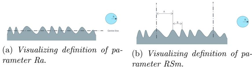
Figure 4.8: *Parameters for defining surface roughness and designing for optimal scratch resistance.*
