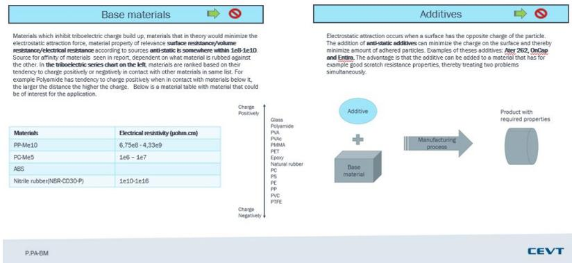
Figure 7.3: Design guideline section prevention particle adhesion with regard to base material.
