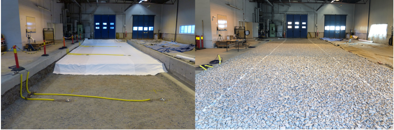
Figure 6.6: The experiment setup before and after filling. The load cells are positioned at the bottom of the channel, and granular material is placed on top with an excavator.
