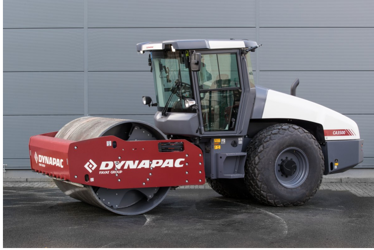
Figure 3.1: Dynapac CA3500D single drum vibratory roller, the machine used in the experiments and modelled in the multibody solver. Reproduced with permission from Dynapac.
