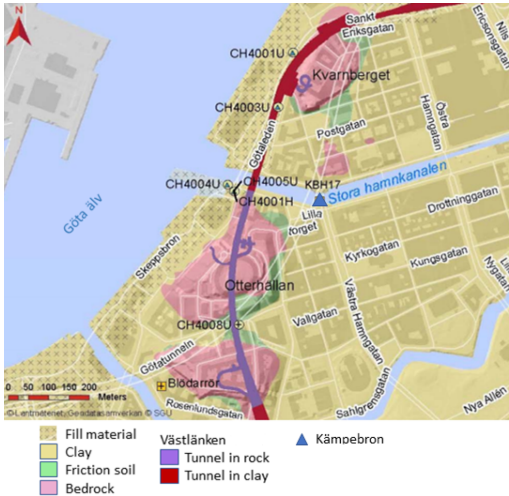
Figure 3.2: Soil map of the studied area, including Västlänkstunneln in rock and soil and Kämpebron. Modified from Trafikverket (2016c).
