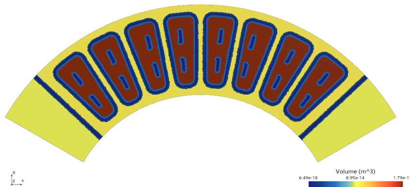
Figure 4.2: Cell Size as a Colour Shaded Plot Looking at the Rotor Surfaces
