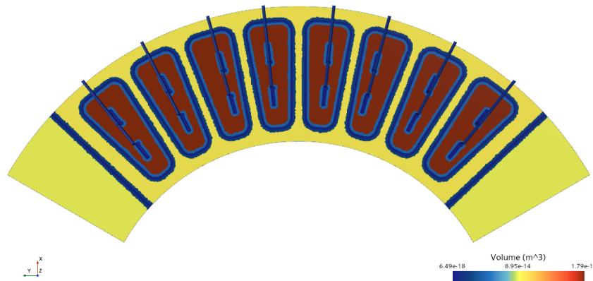
Figure 4.1: Cell Size as a Colour Shaded Plot Looking at the Stator Surfaces
