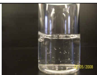
Figure 43. A solution of 15 mM dodecyl glutamate at pH 6.14, small precipitates can be seen.
