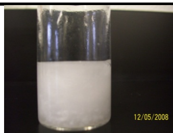
Figure 46. A solution of 15 mM dodecyl glutamate At pH 5.12, the solution is now very cloudy from the precipitation.
