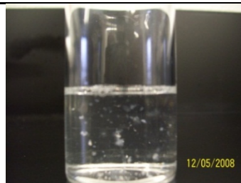
Figure 44. A solution of 15 mM dodecyl glutamate at pH 5.55, the precipitates are getting larger.
