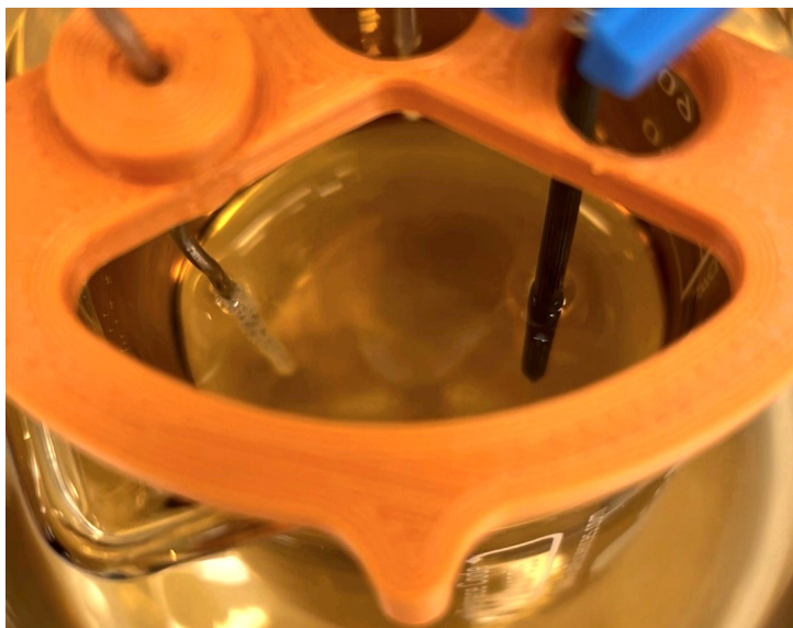
Figure 4.1: Pt (left) & graphite (right) electrode in 0.5 M \text{H}_2\text{O}_2 solution. Possible \text{O}_2 bubbles are visible on Pt.
