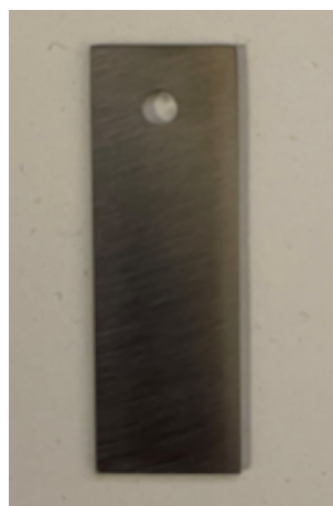
Figure 3.2: a) Schematic of sample. b) Image of Zry2-sample after preparation.
