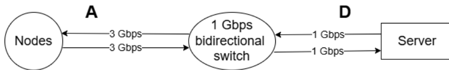
Figure 4.4: A simplified network model where link A represents the aggregated bandwidth between all nodes and the switch. Link D is between the server and the switch.
