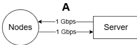
Figure 4.5: A minimal network model where link A represents the whole network, clarifying the 1 Gbps bottleneck imposed by the link to the server.
