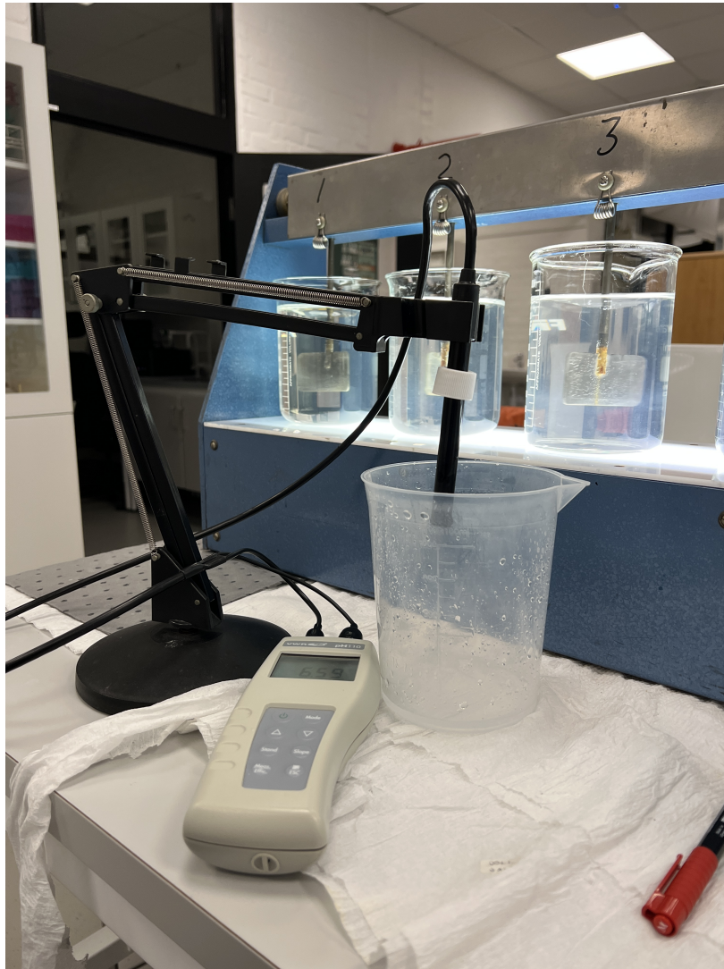
Figure 4.3: pH meter being used to measure the pH of water samples during a Jar Test.
