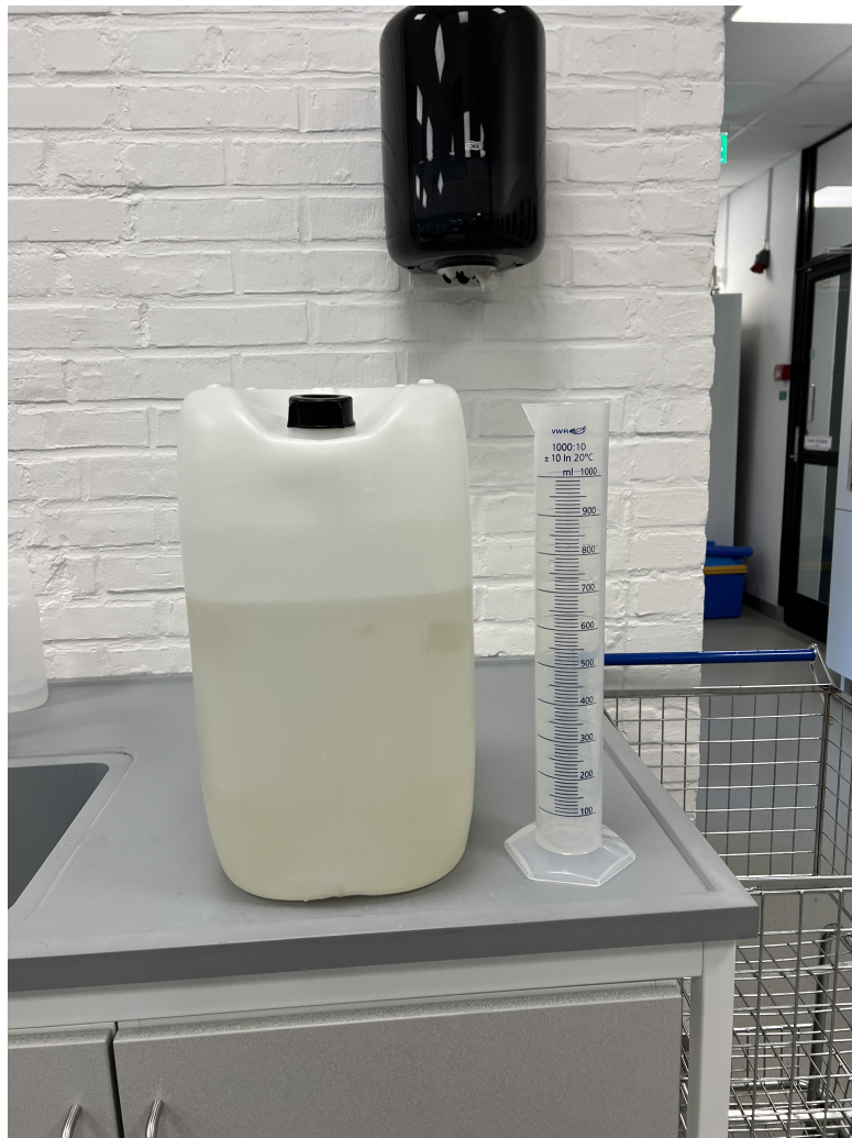
Figure 4.1: Setup used to measure 900 ml of water in beakers for a jar test. A 25 L can of raw water and a 1000 ml measuring glass are shown in the figure. The setup is simple and efficient, ensuring that the correct volume of water is added to each beaker, which is crucial for accurate test results.
