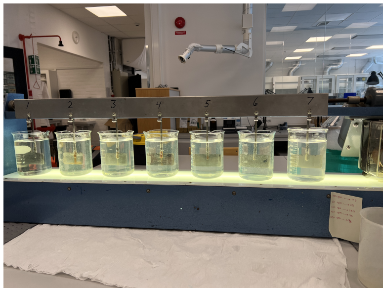
Figure 4.2: Experimental setup for the Jar Test. Seven large beakers with a capacity of 1000 ml each are arranged in a row on a stirrer.
