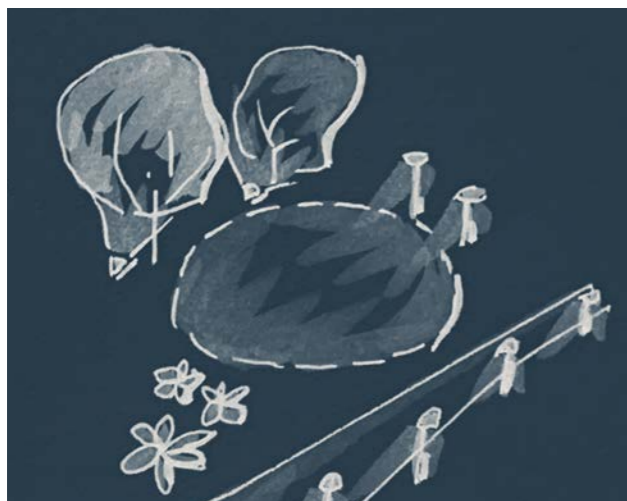
Carefully placed lightning, not too much light Not dazzling, use light close to the ground Set light on objects
