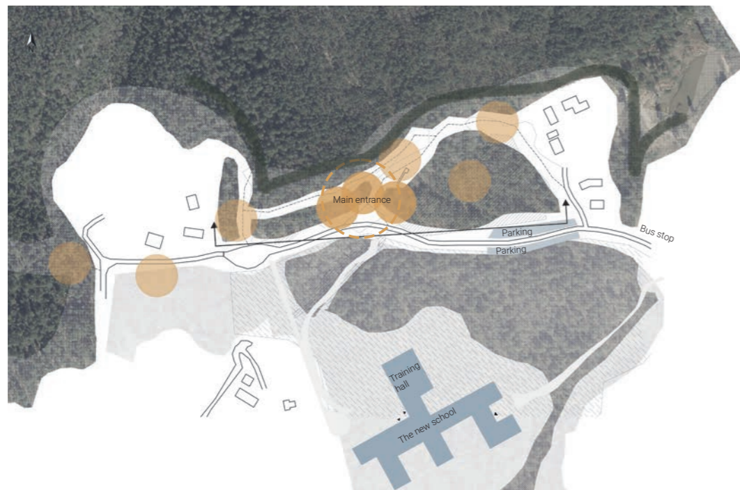
An early concept sketch showing the relationship to the new school planned by the municipality. To lower the amount of traffic passing by the trail centre, the parking can be relocated from the proposed one to this where it is placed along the side of the road closer to the bus stop. No scale.
