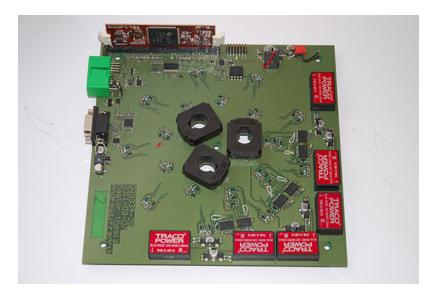
Figure 13: The finished populated controller PCB
