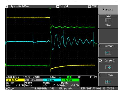
Figure 28: Induced oscillations on 5V supply. Ch1: Source-Drain on upper MOSFET, Ch4: Source-Drain on lower MOSFET and CH3: 5V supply line.
