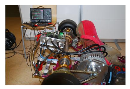
Figure 14: Picture showing the complete driveline with the inverter
