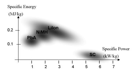
*Figure 12. Specific power and energy for different ESS technologies.*
