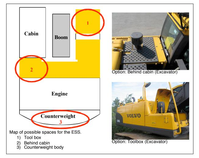
*Figure 17. Detailed pictures of the possible locations of ESS in the excavators.*
