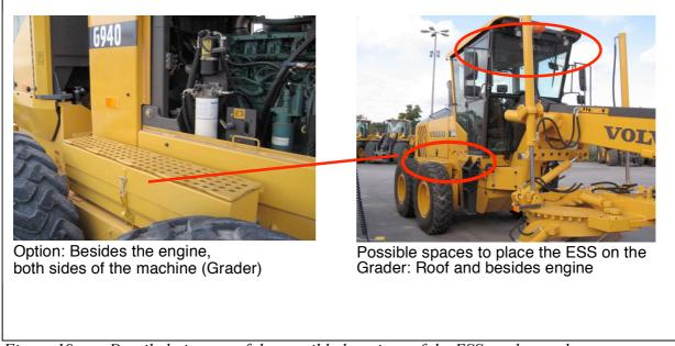
*Figure 19. Detailed pictures of the possible locations of the ESS on the grader.*
