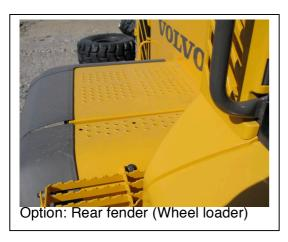
*Figure 18. Detailed picture of the possible location of ESS on the wheel loader.*
