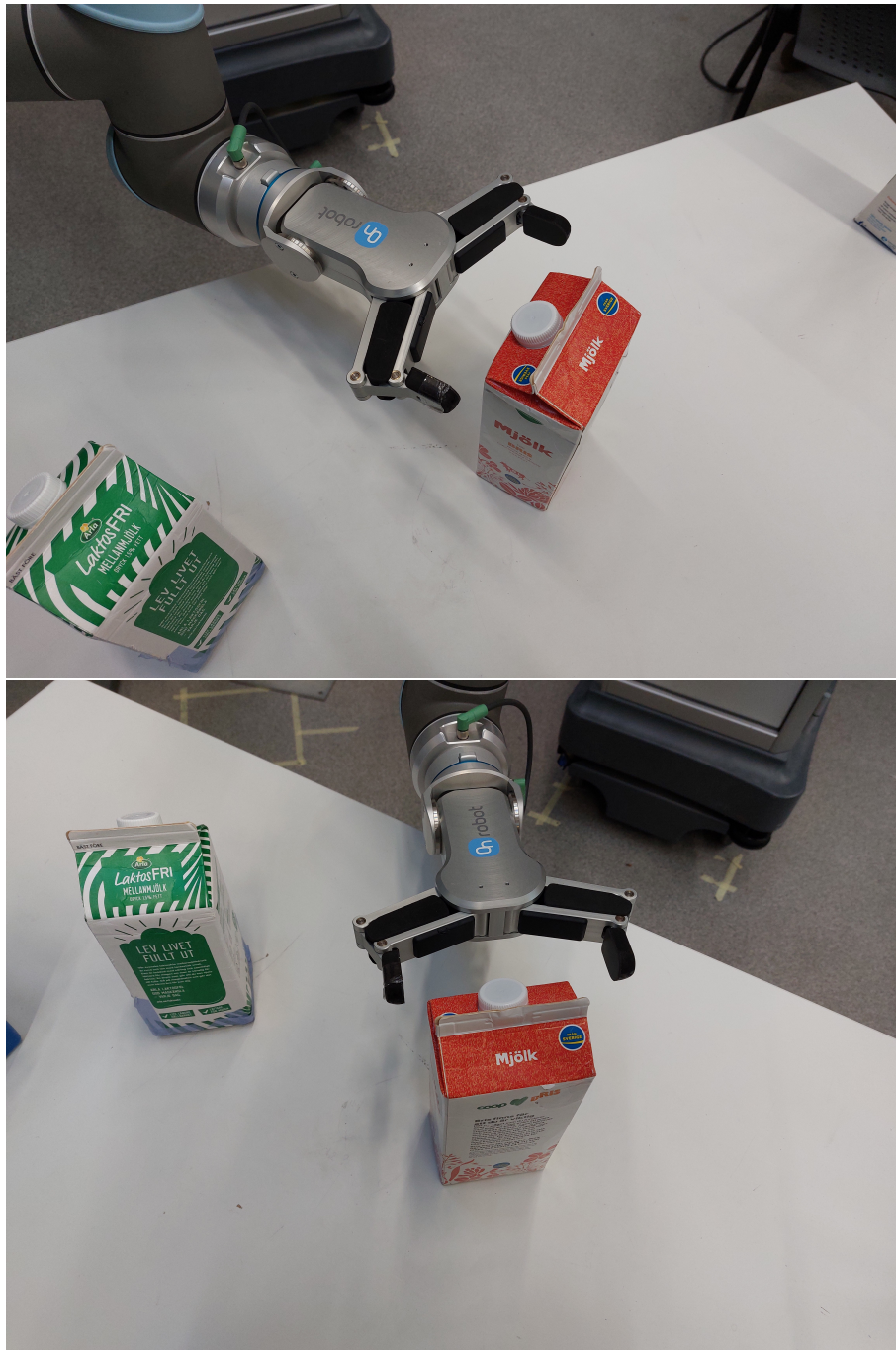
Figure 7.6: Gripper pose after reaching the grasp pose from two standpoints
