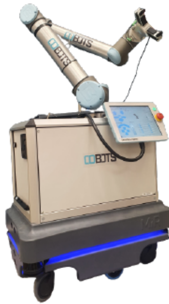
Figure 3.6: The mobile manipulator used in this work. The mobile base is MIR200, the arm is UR10 and the gripper is OnRobot RG6
