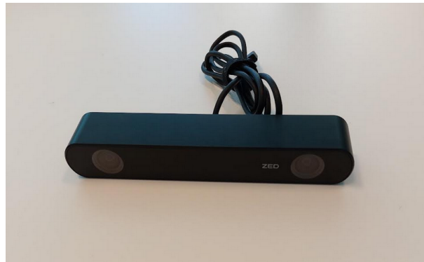
Figure 3.3: ZED2 Camera from Stereolabs
