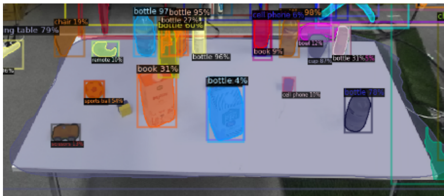
Figure 5.3: Image segmentation generated by Mask-RCNN with a low threshold
