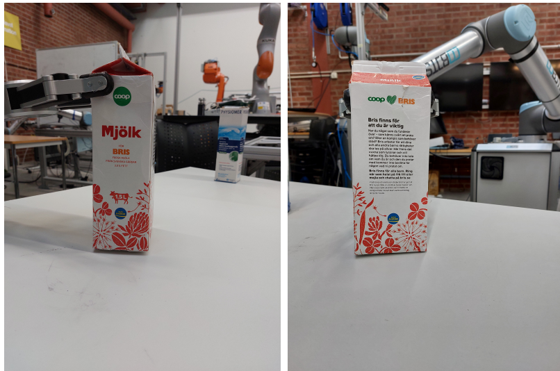
Figure 7.7: Pose of the fingers when the object is grasped by the robot
