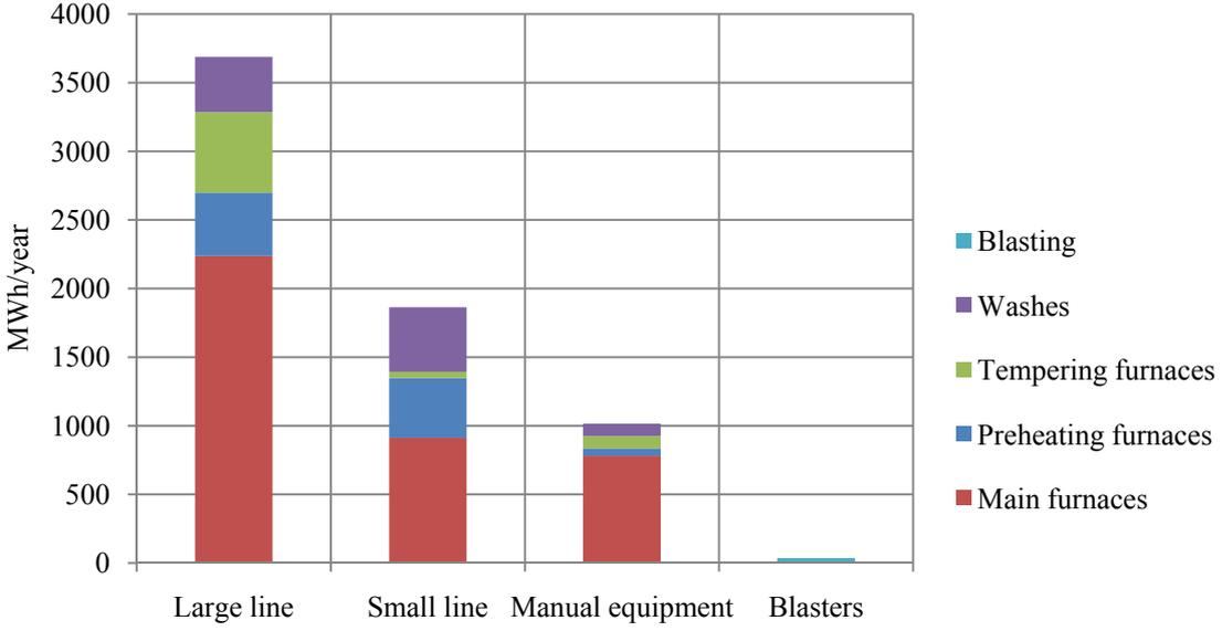
Figure 15. Distribution of the energy usage in the process during one year in MWh.
