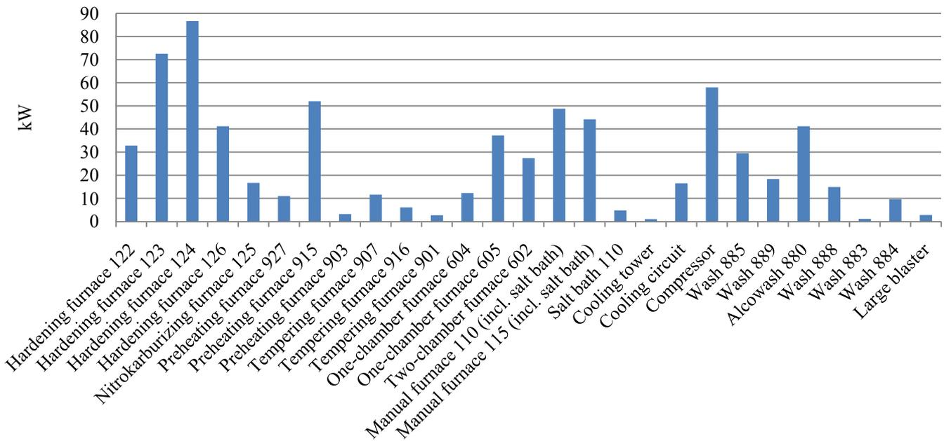
Figure 18. The mean power load in kW for the process equipment.
