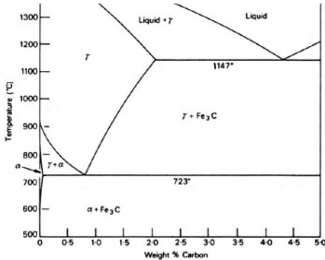
Figure 1. Phase diagram for iron-carbon alloys.
