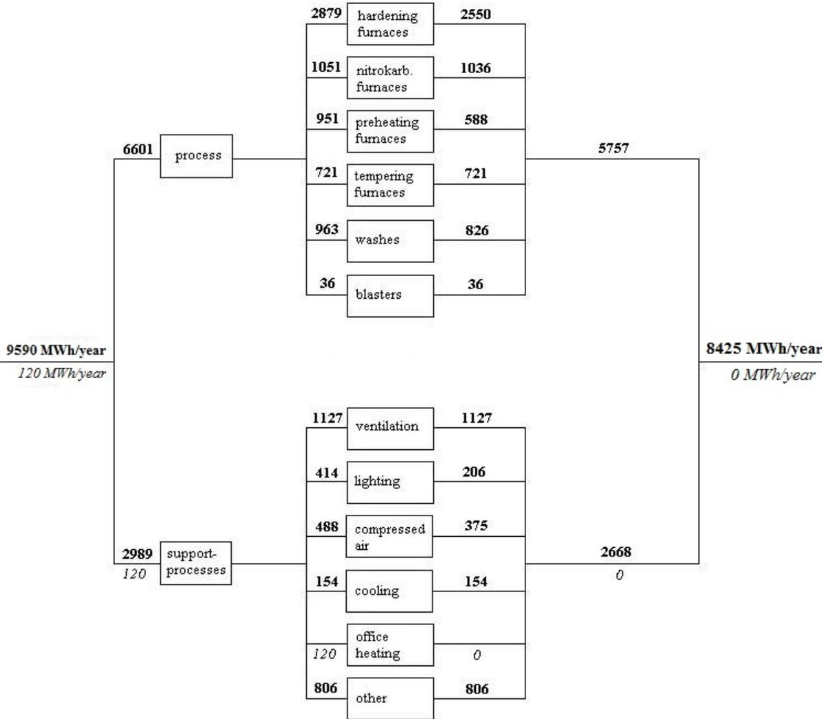
Figure 23. The energy consumption distribution in MWh/year in the plant at the start of the project and after implementation of case III presented as a fish bone diagram. The numbers in bold are electricity demand and the numbers in italic are district heating demand.
