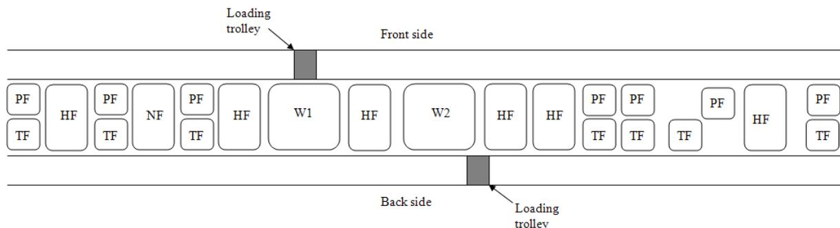
Figure 7. An overview of the large line of furnaces, where PF stands for preheating furnace, TF for tempering furnace, HF for hardening furnace, NF for nitrocarburizing furnace and W1 and W2 for washes.
