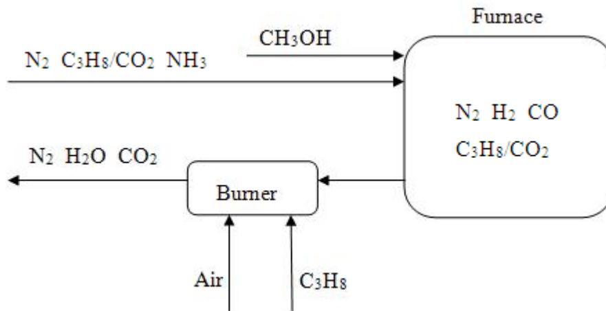
Figure 5. The gas flows in a heat treatment furnace.
