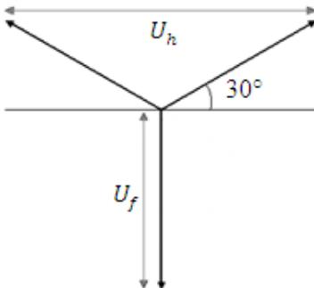
Figure 3. The relationship between the phases and the voltages where  $U_h$  is the principal voltage and  $U_f$  is the phase voltage.
