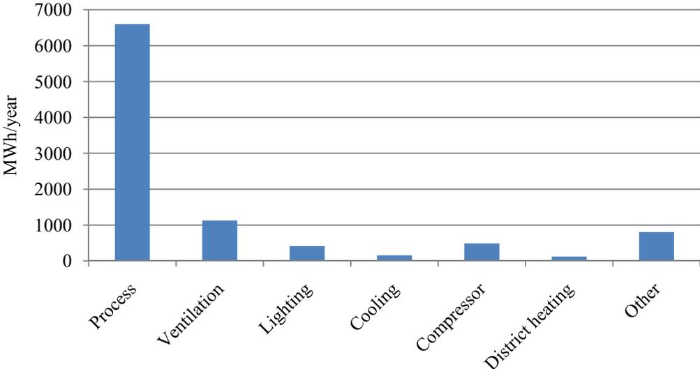
Figure 14. Distribution of the energy usage during one year in MWh.
