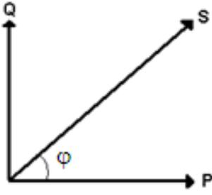
Figure 4. The relationship between the power loads where  $S$  is the apparent power load,  $P$  is the active power load and  $Q$  is the reactive power load.
