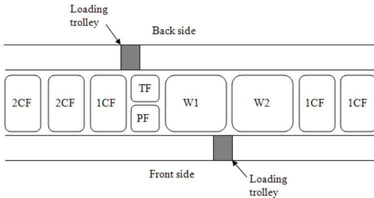
Figure 8. An overview of the small line of furnaces, where PF stands for preheating furnace, TF for tempering furnace, 1CF for one-chamber furnace, 2CF for two-chamber furnace and W1 and W2 for washes.
