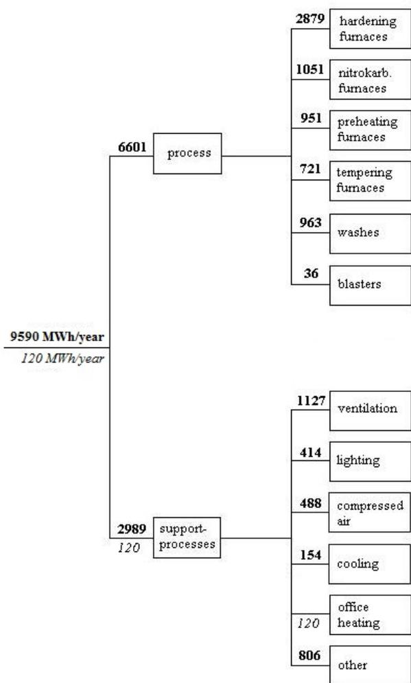
Figure 16. The energy consumption distribution in MWh/year in the plant presented as a fish bone diagram. The numbers in bold are electricity demand and the numbers in italic are district heating demand.
