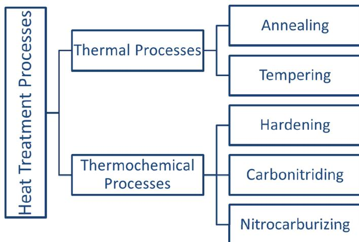
Figure 2. Categorization of heat treatment processes.
