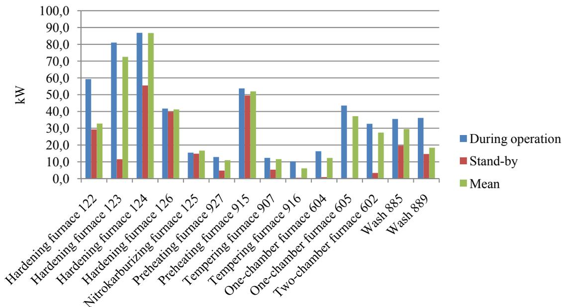
Figure 19. The power load in kW during operation and in stand-by for the process equipment.
