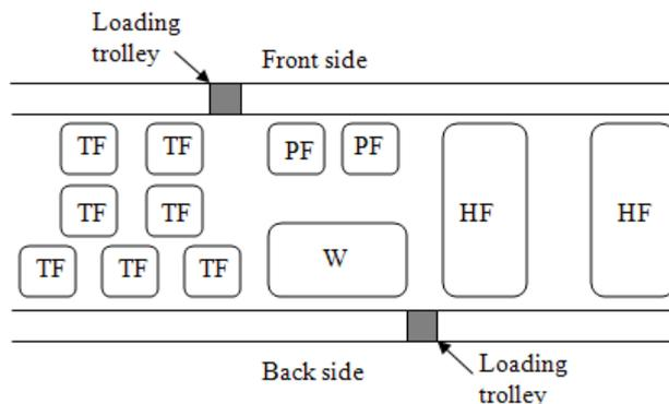
Figure 9. An overview of the manually operated furnaces, where PF stands for preheating furnace, TF for tempering furnace, HF for hardening furnace and W for wash.
