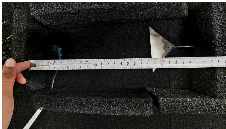
Figure 3.3: Corner Reflector placed at approximately 23.5 cms from the Radar
