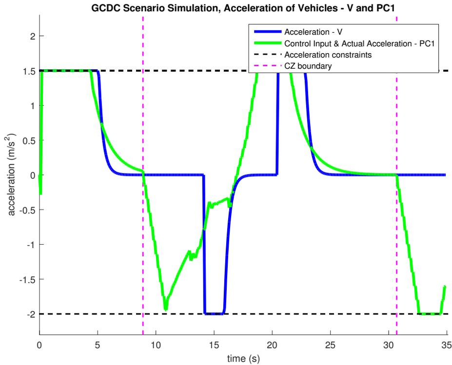
**Figure 5.1:** Acceleration of  $PC1$  ( $U_2(k)$ ) when  $\hat{U}_{1,constant} = u_{min}$
