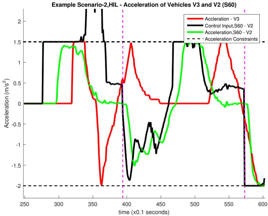
**Figure 6.12:** Acceleration of  $V_2$  and  $V_3$  - Example Scenario 2, HIL
