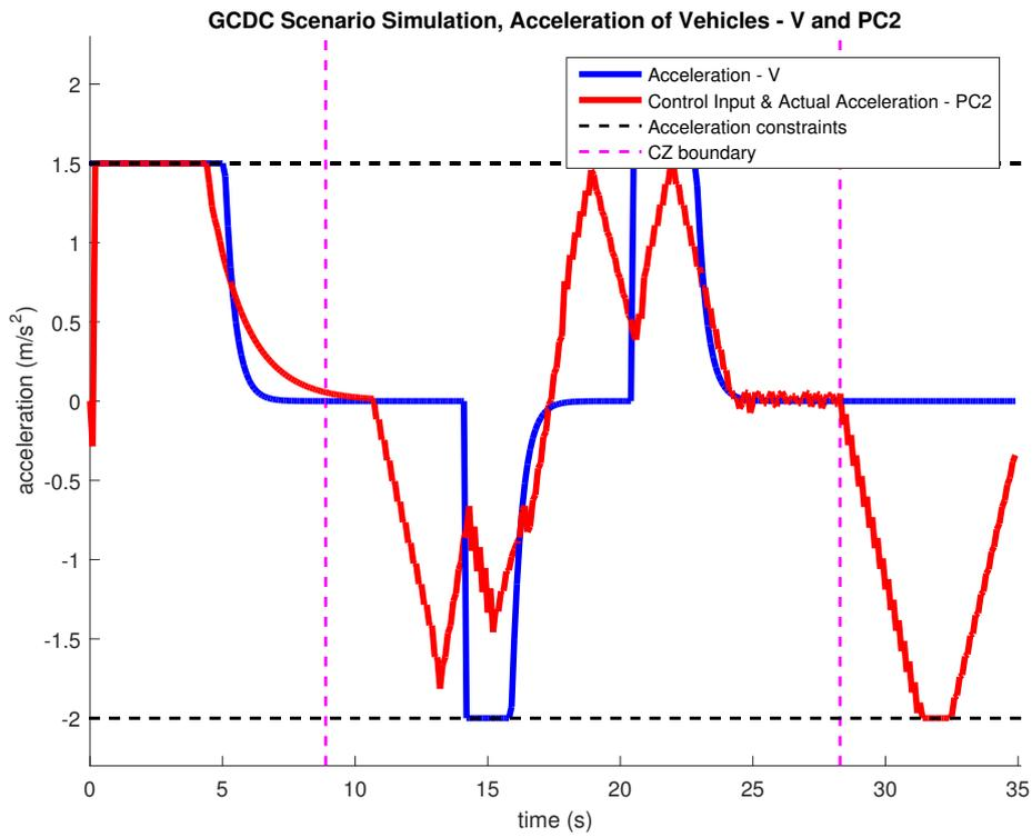
Figure 5.4: Acceleration of *PC2* inside CZ
