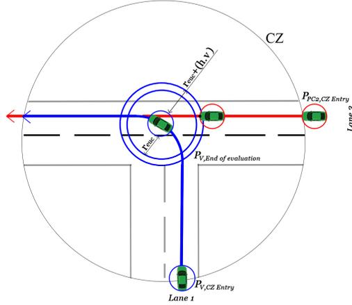
**Figure 3.3:**  $PC_2$  Position Constraints - GCDC Intersection Scenario
