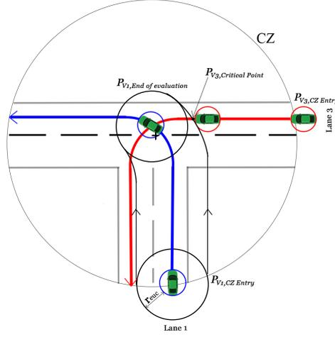
**Figure 3.5:**  $V_3$  Position Constraints of Example Scenario 2
