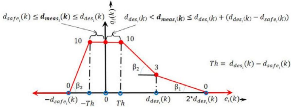
**Figure 2.6:**  $Q_2$  Desired Distance Scoring Function (www.gcdc.net)
