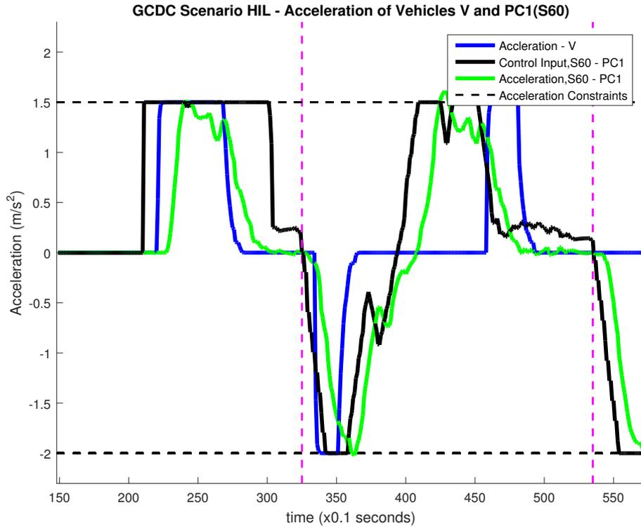
**Figure 6.3:** Acceleration of  $V$  and  $PC_1$  - GCDC Scenario HIL
