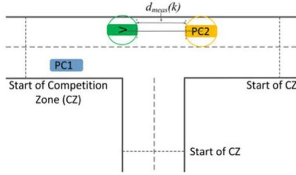
**Figure 2.5:** Desired Distance between  $V$  and  $PC_2$  (www.gcdc.net)
