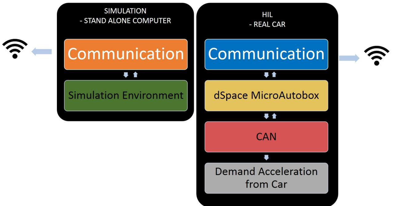
**Figure 6.1:** Hardware In Loop (HIL) Simulation Scheme
