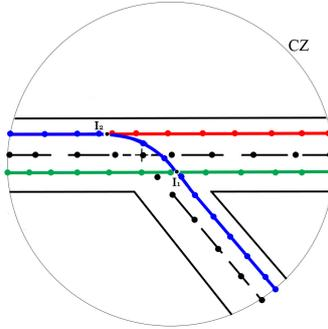
**Figure 4.2:** Trajectories definition from Recorded GPS data
