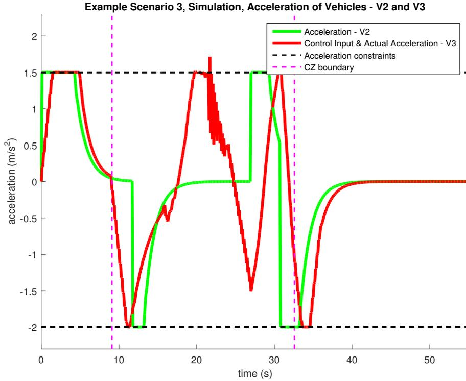
**Figure 5.13:** Acceleration of  $V_2$  and  $V_3$  - Example Scenario - 3
