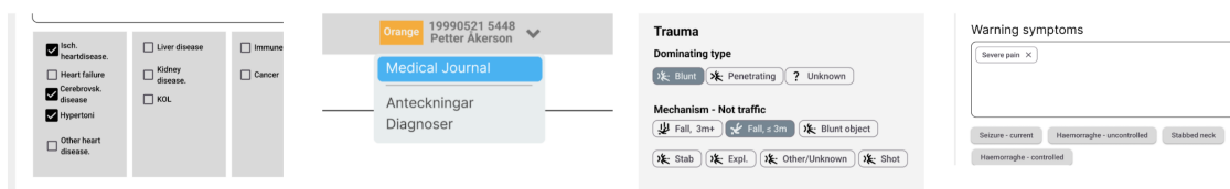
Figure 5.13: Example of option picker solutions. From left: Checkboxes, Dropdown menu, Two versions of input chips
