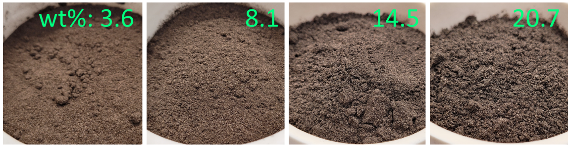
Figure 5: Four different samples after granulation using BaM. The PVA solution content in wt% is displayed in the green text.
