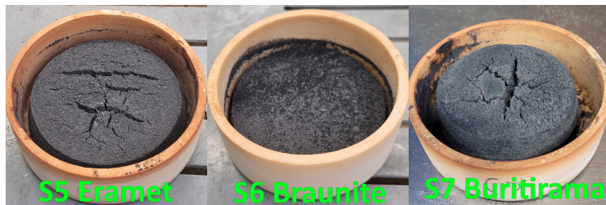
Figure 8: Three samples after sintering. The samples are made from different manganese ores and where sintered at different temperatures. Samples left to right: S5 is eramet ore at 1215 °C, S6 is braunitz ore at 1215 °C, S7 is buritirama ore at 1265 °C
