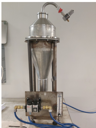
Figure 3: Picture of the customized jet rig which is used to perform the attrition test on the particles.
