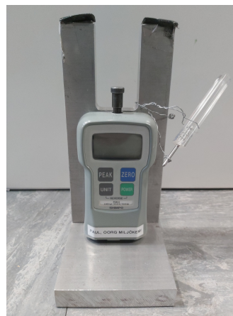
Figure 4: Picture of the crushing strength apparatus with the needle hanging to the right.
