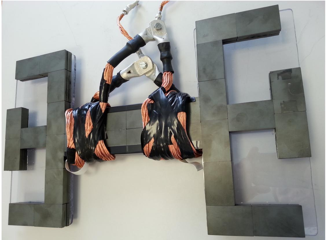
Figure 4.18: The coils and ferrites.
