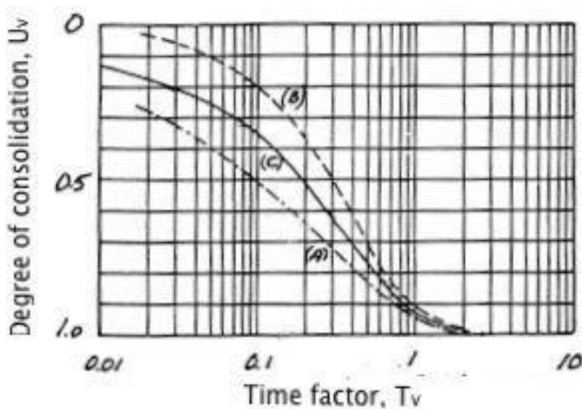
Figure 5-4 Time factor and degree of consolidation (Sällfors, 2009).
