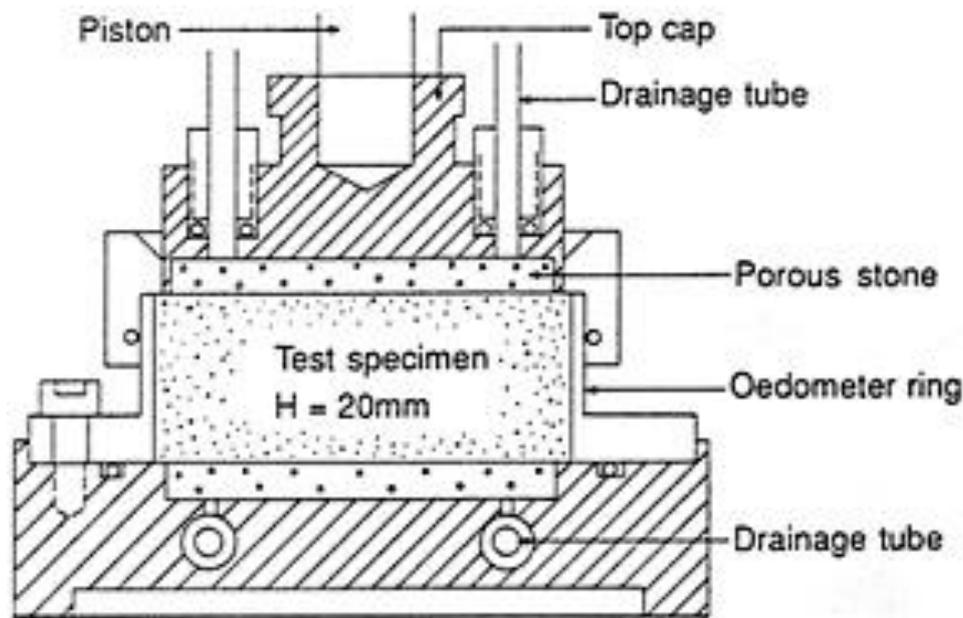
Figure 2-6 Schematic drawing of oedometer (NGI, 2014)/
