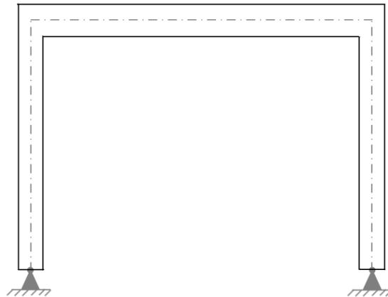
Figure 3.2: System drawing of the modelled boundary conditions of the bridge
