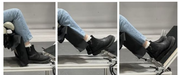
Figure 10. Testing in driving position, only lower leg support and both lower leg support and footrest.
