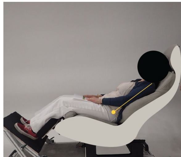
Figure 55. Freely chosen torso angle (test person seated with leg and foot support (1)).
