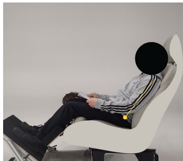
Figure 56. Freely chosen torso angle (test person seated with leg and foot support (2)).
