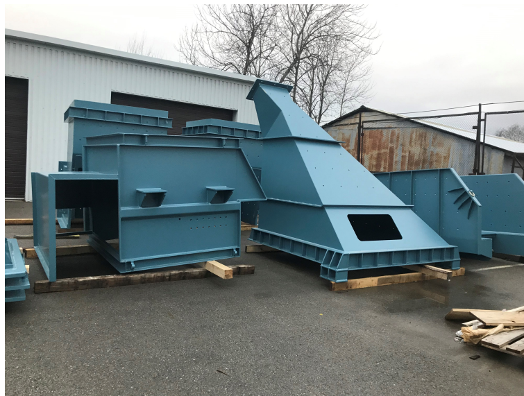
Figure 3.3: Parts of the measuring pocket. Reproduced by permission from ABB
