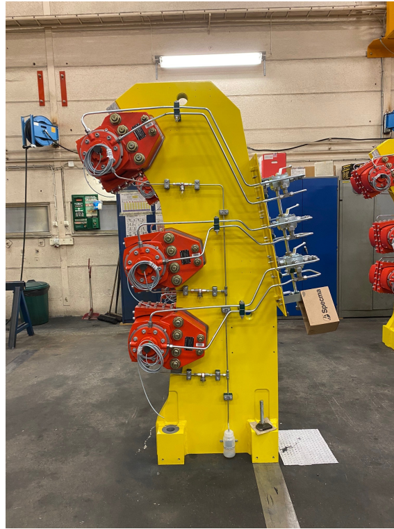
Figure 3.6: Brake stand with associated brake calipers. Reproduced by permission from ABB
