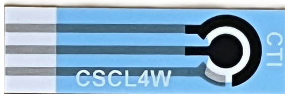
Figure 2.6: Screen printed carbon electrode (SPCE) used in this study, showing the working, counter and reference electrodes.
