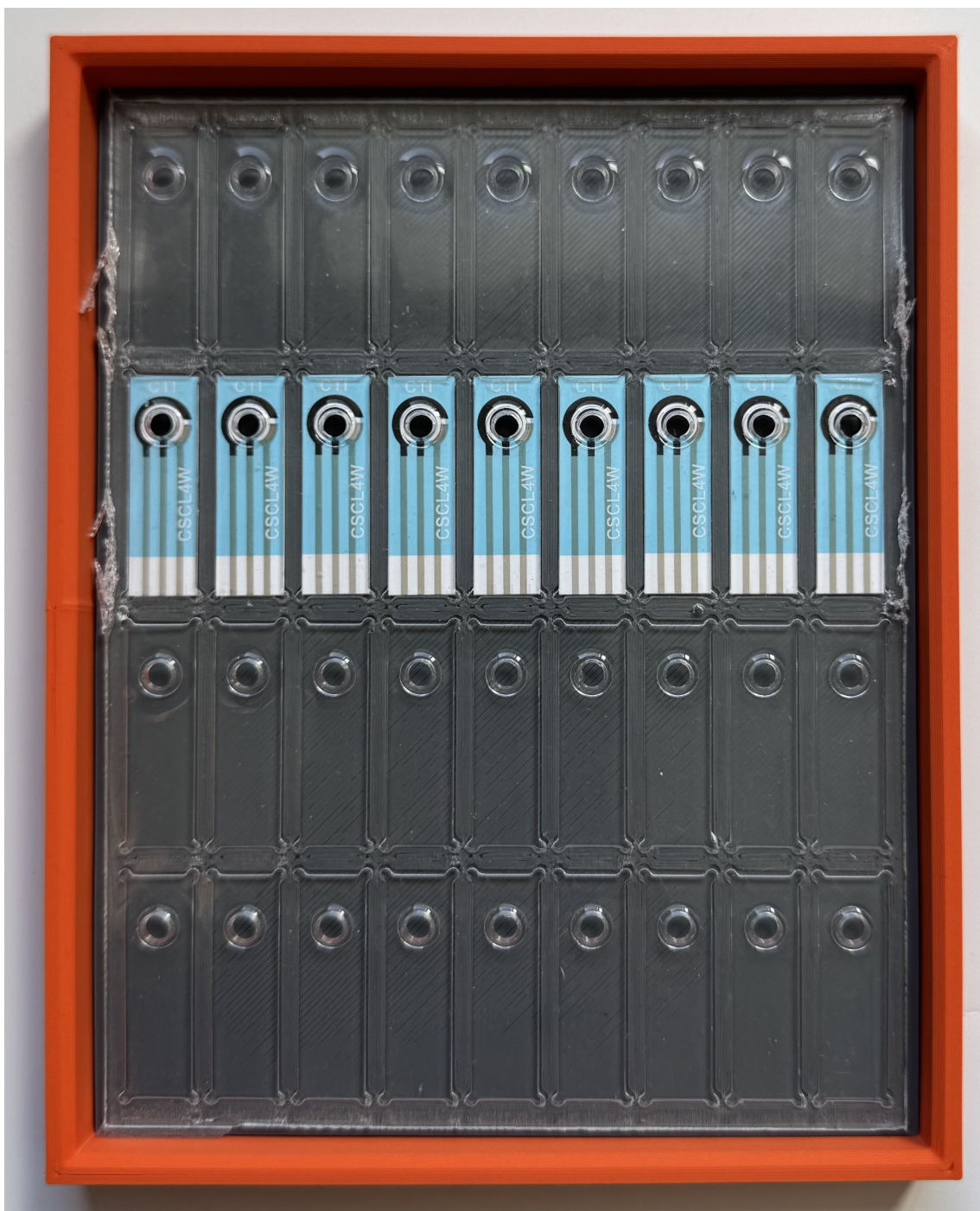
Figure 4.4: 3D printed base plate and frame with carbon electrodes in PDMS.
