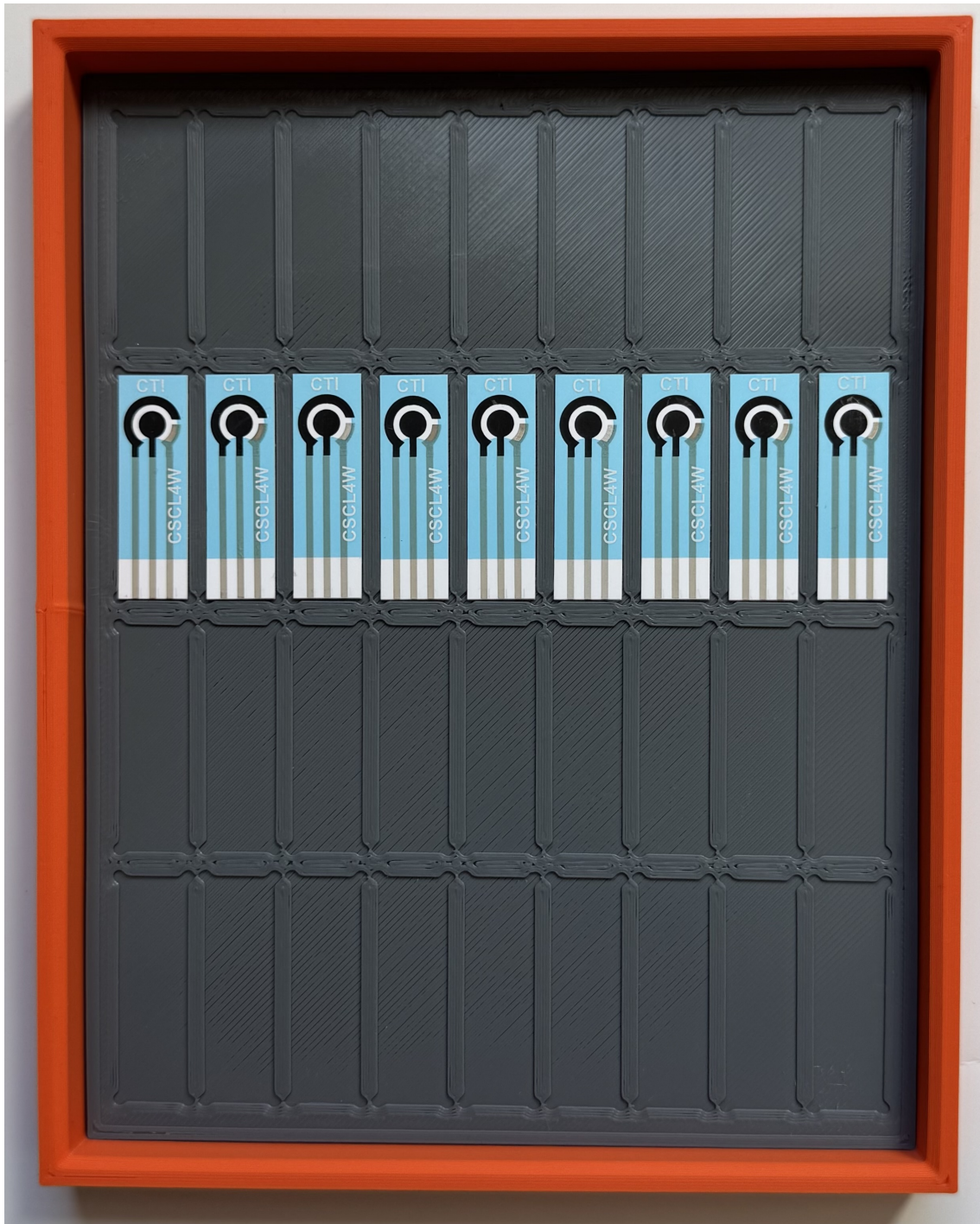
Figure 4.3: 3D printed base plate and frame with carbon electrodes.
