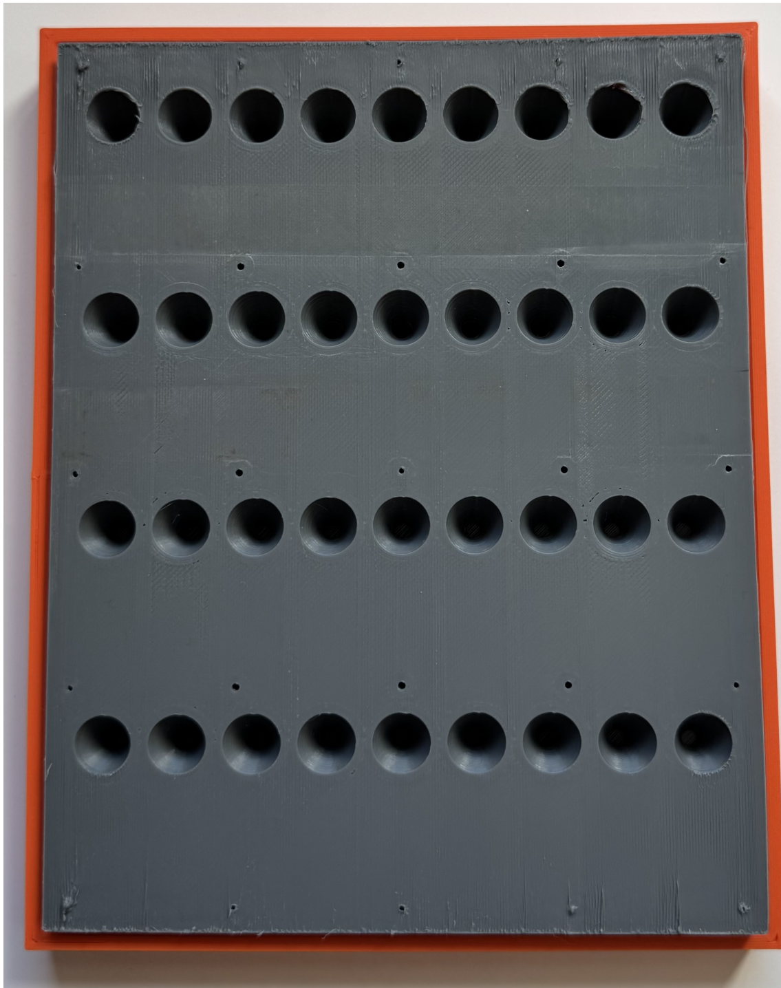
Figure 4.5: 3D printed base plate, frame and top plate with carbon electrodes in PDMS.
