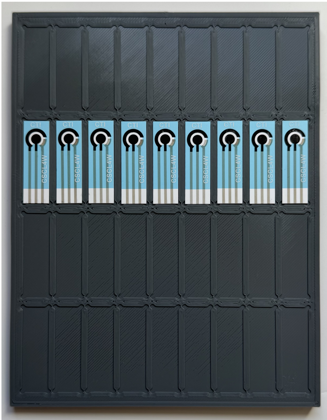
Figure 4.2: 3D printed base plate with carbon electrodes.
