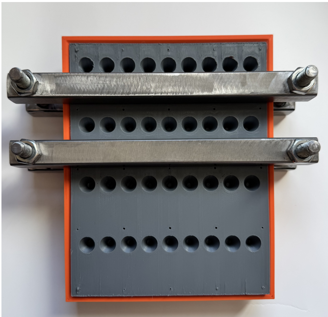
Figure 4.6: Complete sealed PDMS setup from above.
