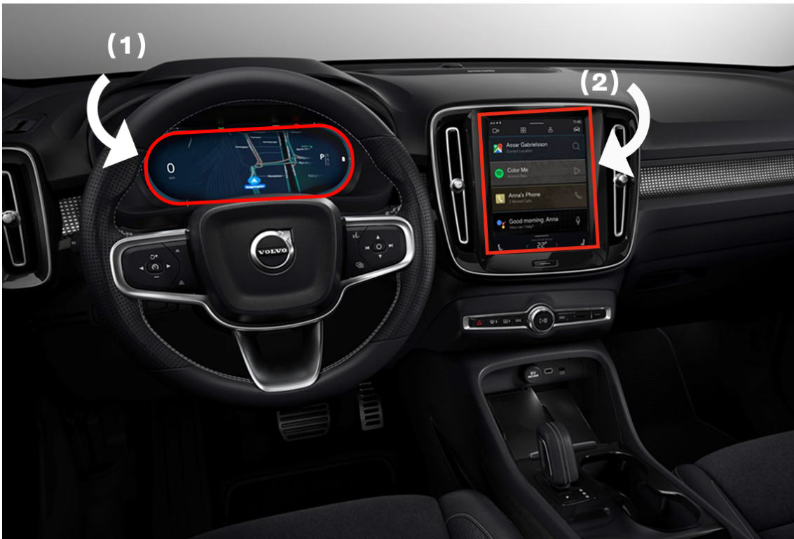
Figure 1.3: Position of the Dashboard Integration Module (DIM) (1) and Centre Stack Display (CSD) (2) in the EV
