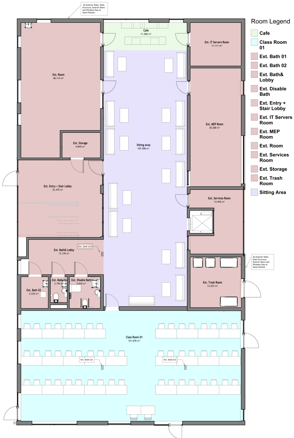
Figure 7 Purposed Layout of Ground Floor HSB Living Lab
