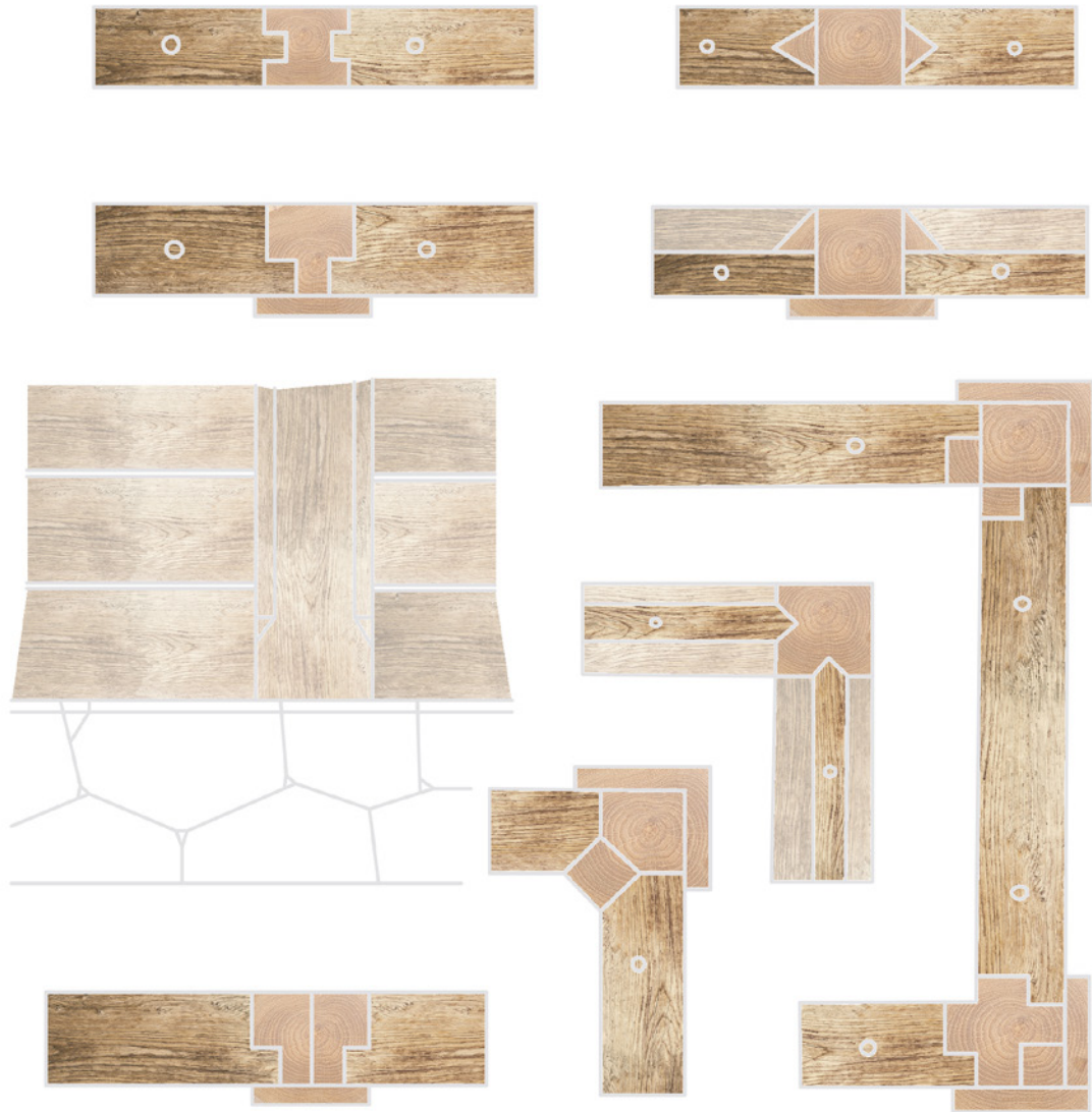
Detail section of various alternative connections between beams and posts, after drawings by Charles Emil Löfvenskiöld in 1868.
