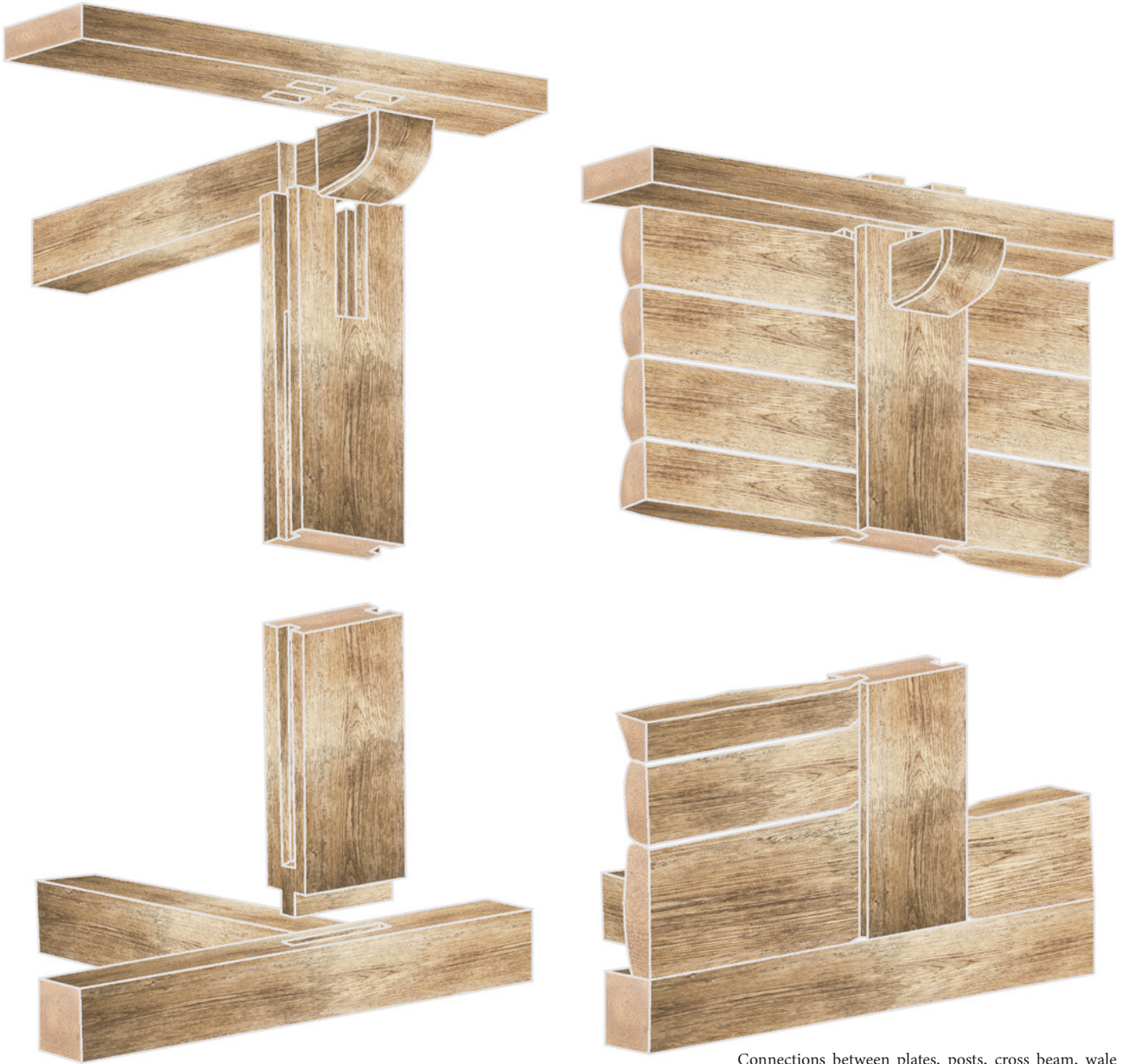
Connections between plates, posts, cross beam, wale and wall planks. The notches of the posts do not go all the way down to the sill plate and the wall planks have chamfered ends that protect the sill plate.
