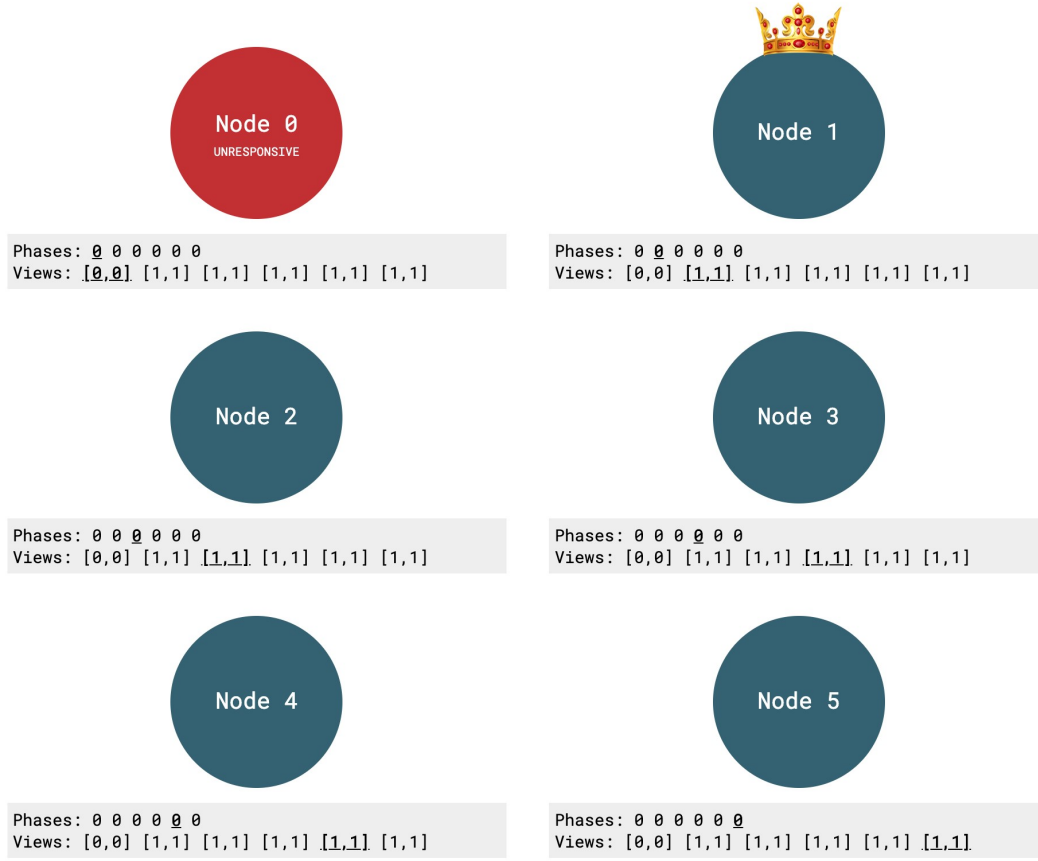
Figure 4.1: A screen shot of the Global view for the View Establishment module. Node 0 is Byzantine and exhibiting a Byzantine behaviour called “UNRESPONSIVE” and processor 1 is the primary, hence the crown. The corresponding view for each processor is shown in the grey box below each processor.
