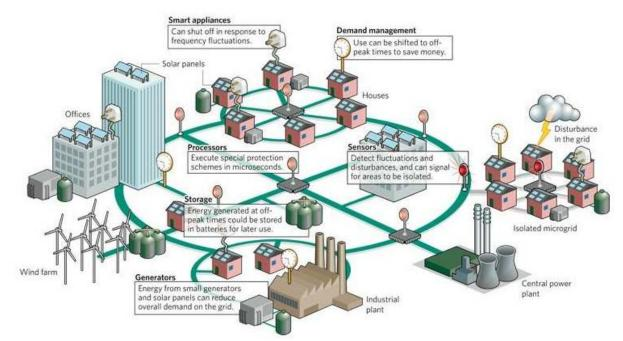
Figure 4 Vision of how a smart grid could look like in the future [18].
