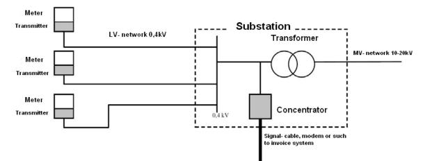
Figure 5 Low voltage PLC communication system.
