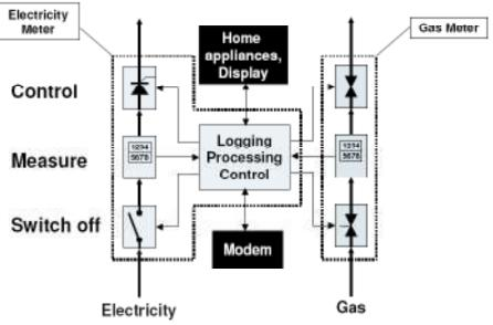
Figure 1 Overview of a smart meter configuration [12].
