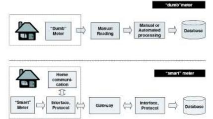
Figure 2 Comparison between an old "dumb" meter and a new "smart" meter [12].
