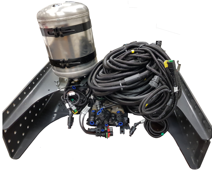
Figure 3.2: Picture showing an example of a fully assembled cross member.
