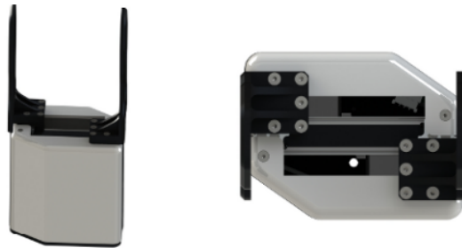
Figure 2.4: TIAGo’s PAL Gripper: Used for Grasping Objects. [[1], p. 21, fig 16. Copyright PAL Robotics]
