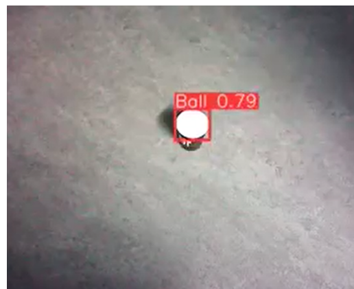
(a) Coffee Mug Placed Close to the Cam- (b) Coffee Mug Placed Far from the Cam- era Detected as "Mug" era Detected as "Ball"
