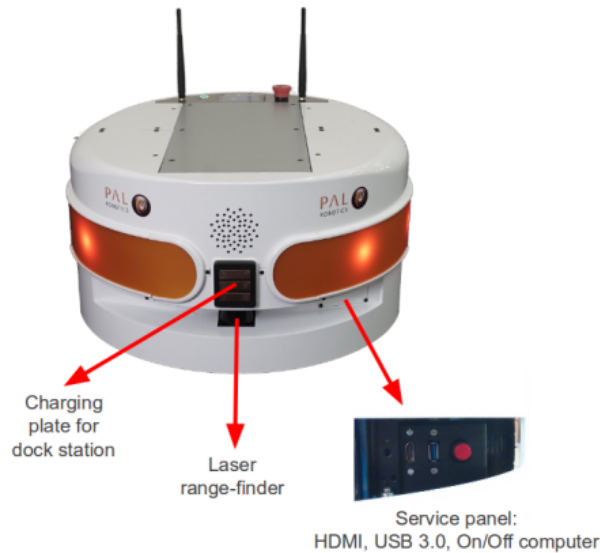
Figure 2.6: TIAGo’s Base for Mobility: Equipped with Sensors for Mapping and Navigation. [[1], p. 10, fig 3. Copyright PAL Robotics]
