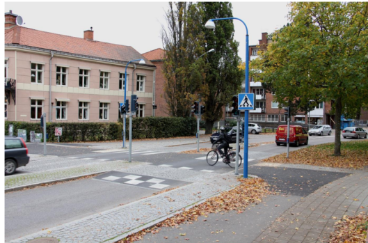
Figure 4.1: Combined crossing on speed bumps. Photo: Eskilstuna kommun
