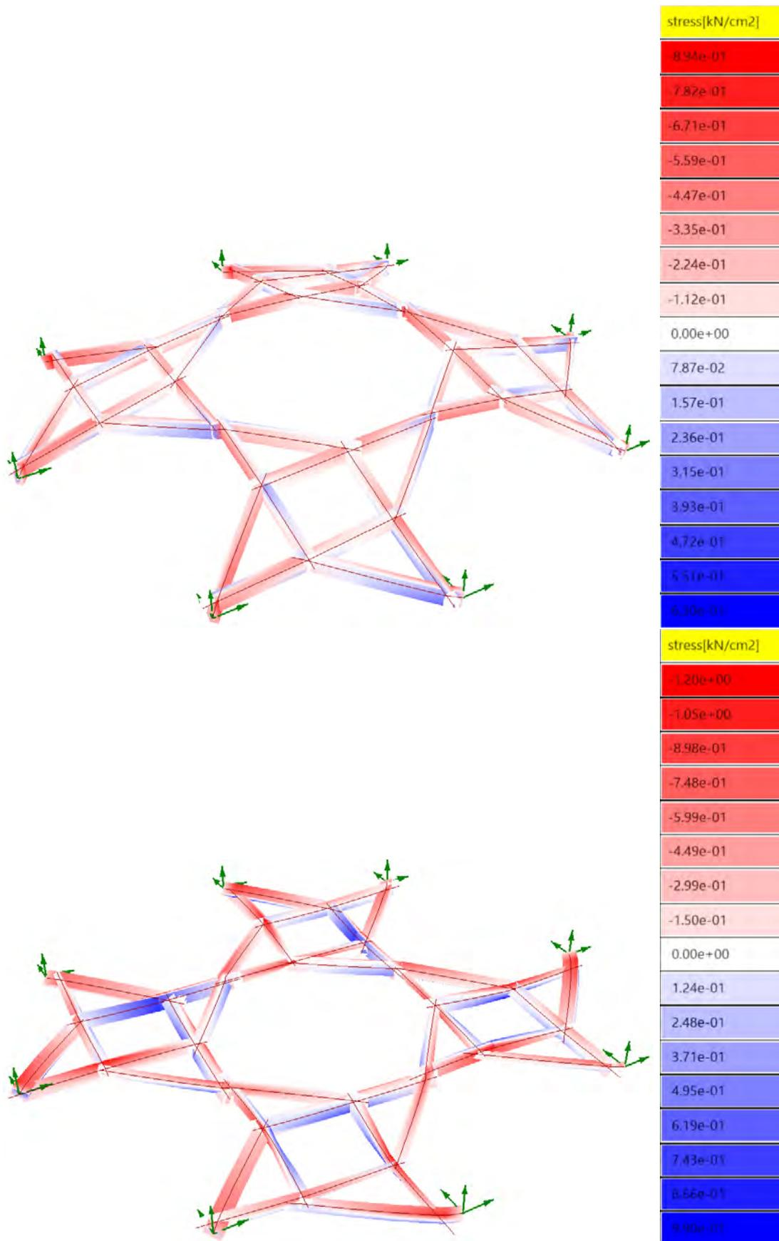
**Figure 6.32:** Axial stress distribution of reciprocal lattice structure from Karamba analysis, rigid connections (left) and semi-rigid connections (right)
