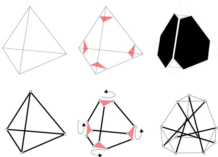
**Figure 3.30:** How to derive a truncated tetrahedron tensegrity geometry based on the tetrahedron geometry
