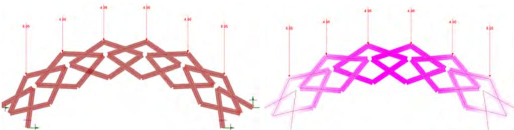
**Figure 6.19:** Symmetric modules in an *arched* line with two supports on each side and a module size of 3.75x1.88 m, *rigid* connections throughout. Undeformed (left) and deformed (right)
