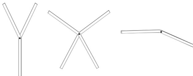
**Figure 3.38:** Scissor modules with angled elements
