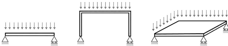
**Figure 3.23:** Section-active structural systems working in tension, compression and bending
