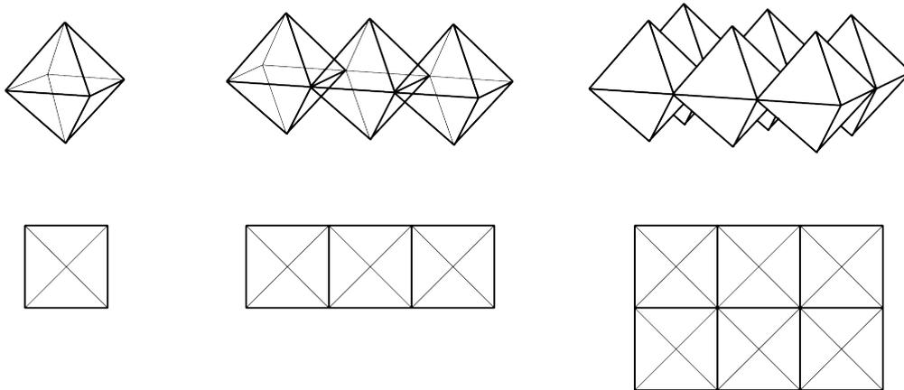
**Figure 4.2:** Octahedrons next to each other can cover a surface due to the square form of the cross-section
