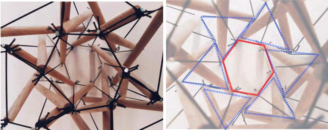
**Figure 4.31:** Zoom in on triaxial weave as tensegrity and basic shapes found in the module
