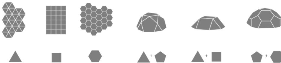
**Figure 5.5:** Examples of geometrical compositions for planar and curved surfaces
