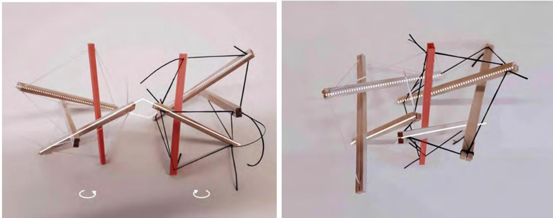
**Figure 4.26:** Weave pattern of two reversed tensegrity modules, one compression element removed when joining
