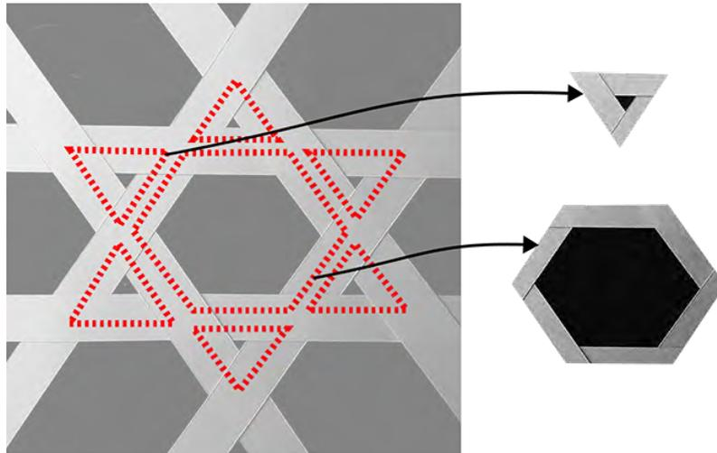
**Figure 4.22:** Zoom of triaxial weave joint, displaying the three- and six-parts of the full module
