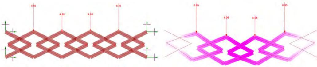
**Figure 6.14:** Symmetric modules in a straight line with two supports on each side and a module size of 3.75x1.88 m, *semi rigid* connections throughout. Undeformed (left) and deformed (right)
