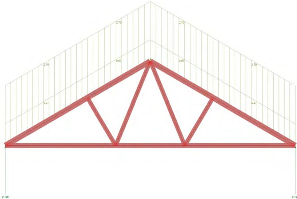
**Figure 6.5:** Standard roof truss from *Swedish Wood* analysed with Karamba
