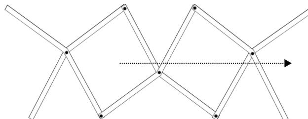
**Figure 3.39:** Angled scissor modules attached to a transverse structure
