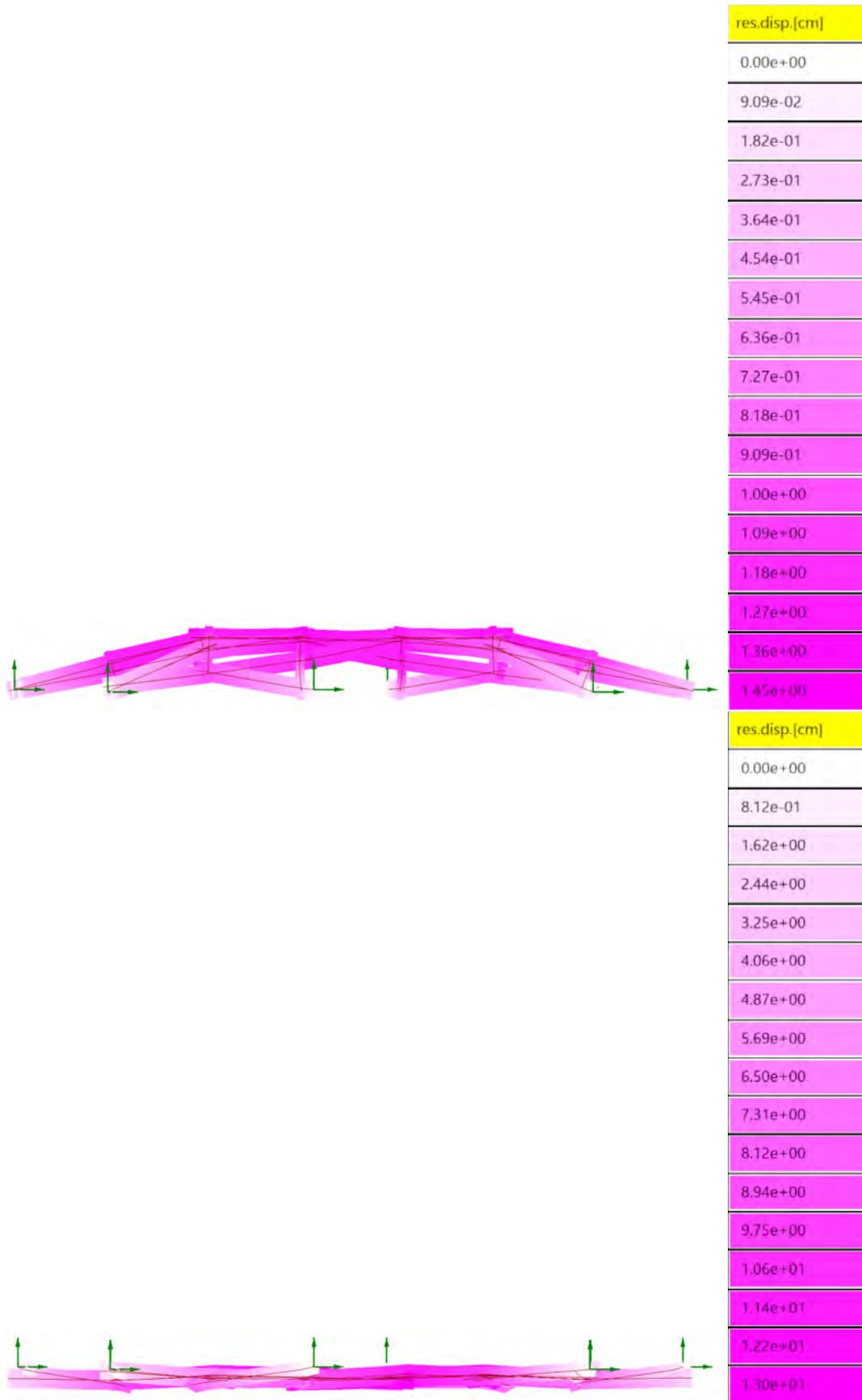
**Figure 6.31:** Deformed model of reciprocal lattice structure from Karamba analysis, rigid connections (left) and semi-rigid connections (right)
