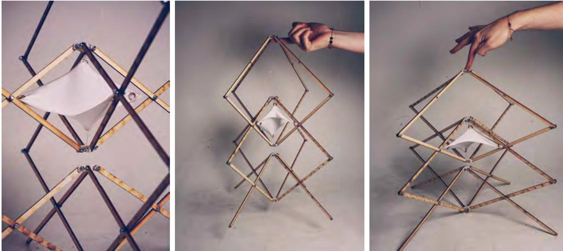
**Figure 4.5:** An elastic piece of fabric works as a tension membrane to stabilise the structure. With the resistance of the piece of fabric added in the middle, the entire structure gain higher resistance to applied loading (image from ArcInTex workshop at NTU, held by Marisela Mendoza).
