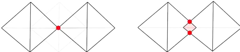
**Figure 5.1:** The connections between octahedron scissor modules; ArchInTex system (left) and octahedron scissor structure (right)
