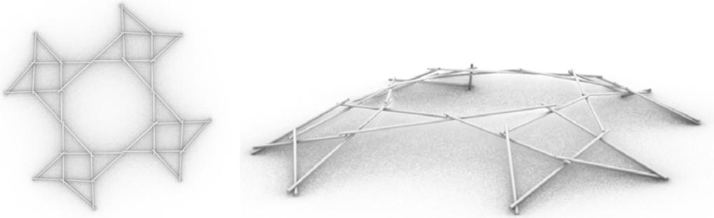
**Figure 5.14:** Digital modelling of the base geometry of a reciprocal lace
