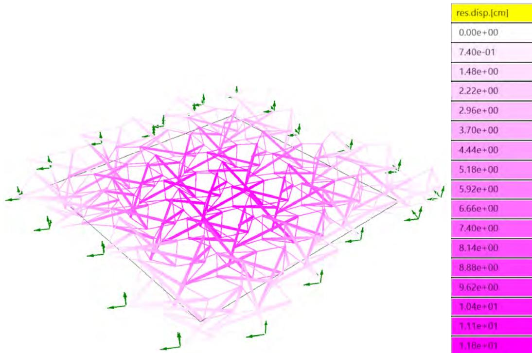
**Figure 6.26:** Deformed model of tensegrity weave structure from Karamba analysis
