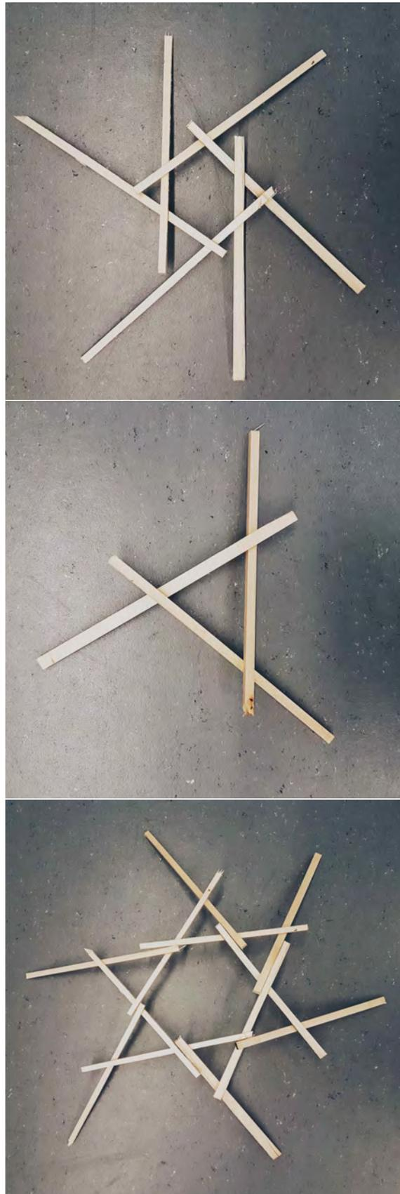
**Figure 4.24:** Triaxial weave as a reciprocal structure
