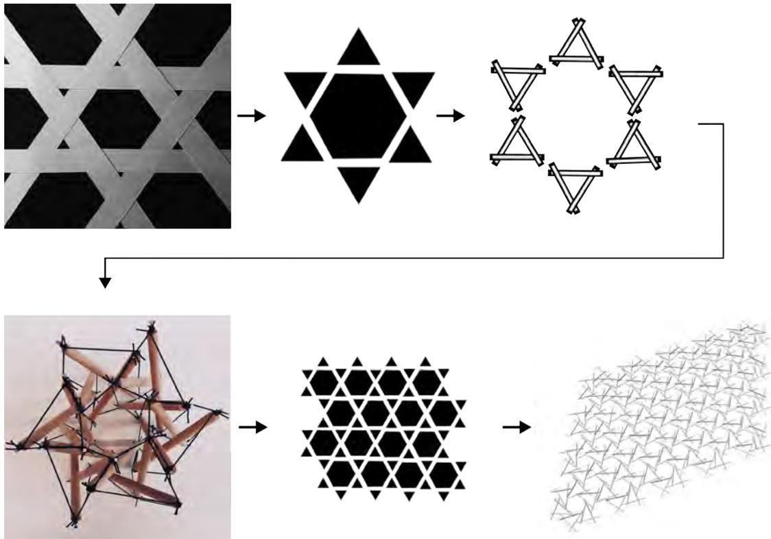
**Figure 1.1:** Method illustration, from the the textile joint to its geometrical interpretation and digital assembly
