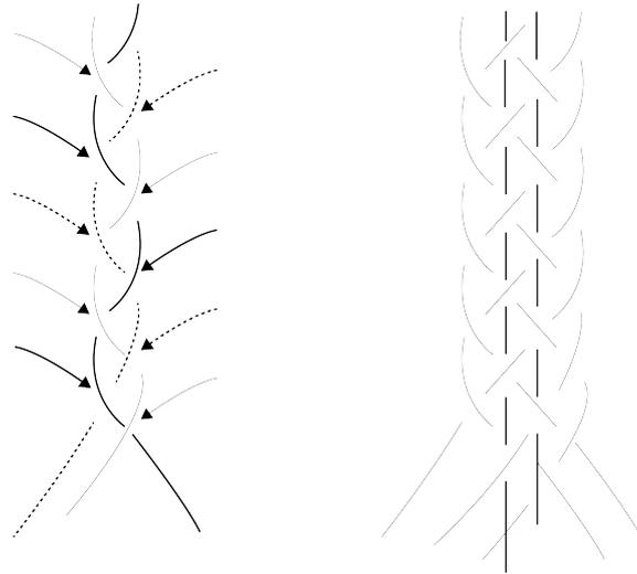
**Figure 3.3:** Left; French braid method, right; inlay yarns in a braid of five yarns
