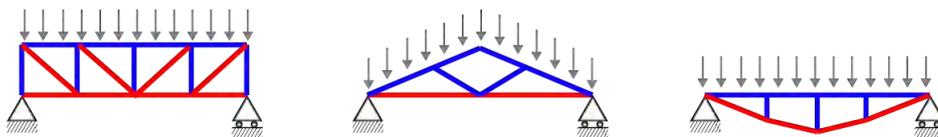
**Figure 3.22:** Vector-active structural systems with members working in pure tension and compression
