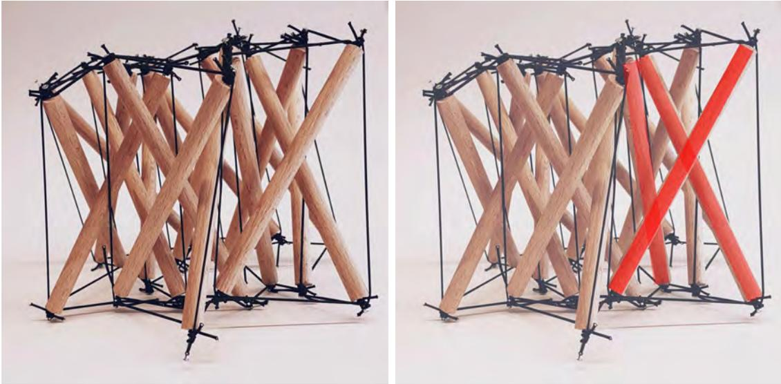
**Figure 4.30:** Triaxial weave binding as tensegrity module, side view
