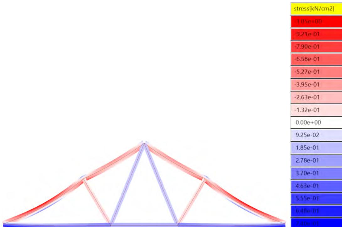
**Figure 6.7:** Axial stress distribution of roof truss analysed with Karamba, the deformation is scaled x10 in the figure
