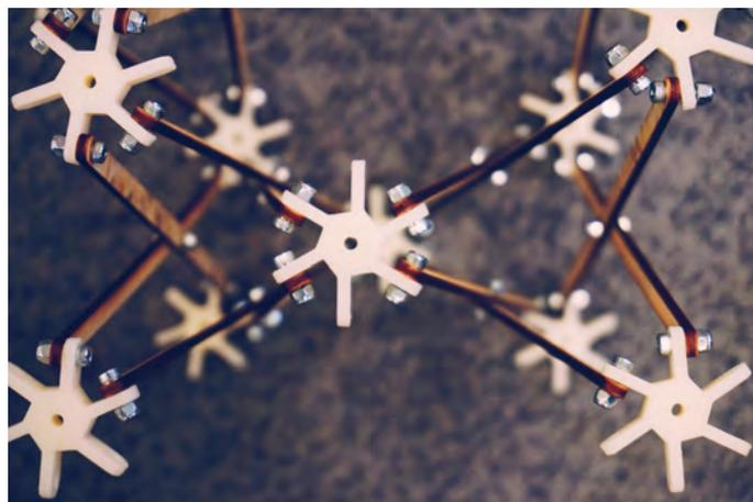
**Figure 3.42:** Three-dimensional joints for scissor structures (image from ArcInTex workshop at NTU, held by Marisela Mendoza)
