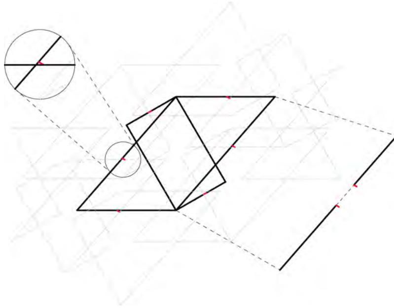
**Figure 5.6:** Modelling of scissor structure; each rod modelled in separate pieces, hinges in red
