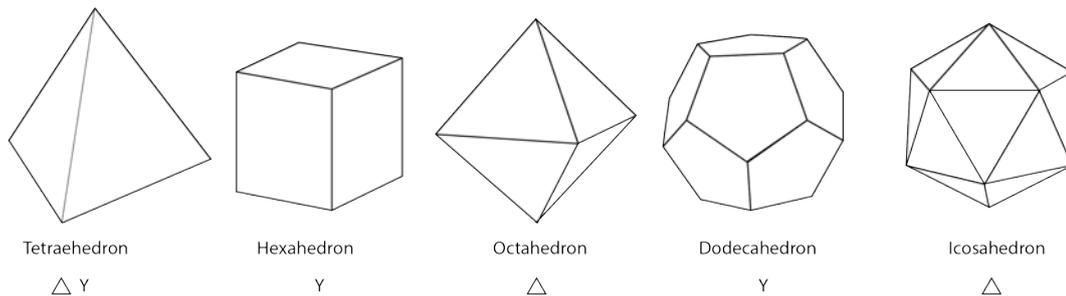
**Figure 3.16:** The five platonic solids. Picture redrawn from *Structural order in space* by T.Wester [19]
