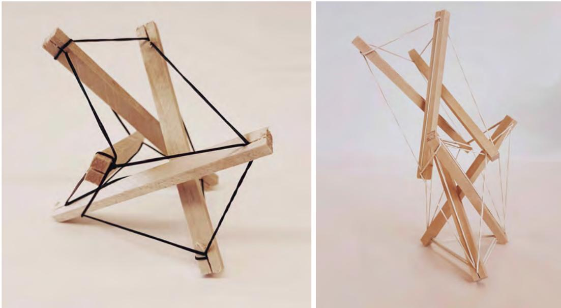
**Figure 4.25:** Tensegrity module and vertical assembly of tensegrity modules
