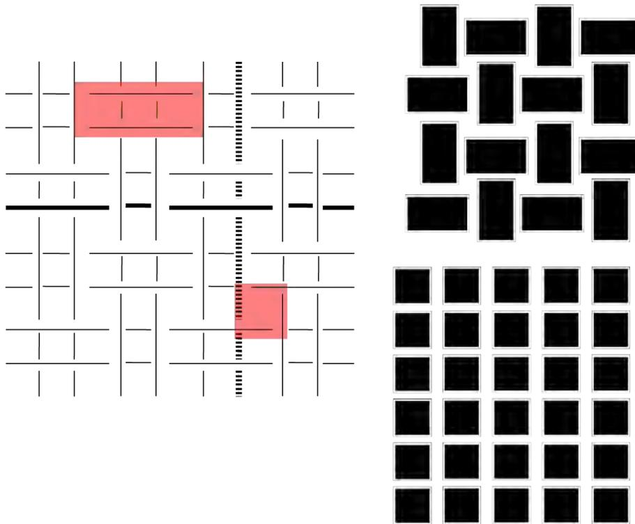
**Figure 4.15:** Geometric interpretation of a double weave, in two different manners
