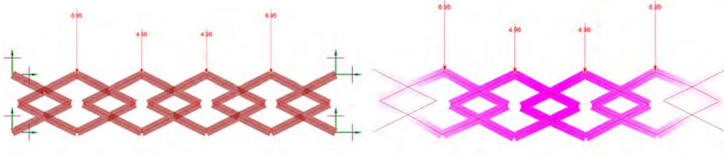
**Figure 6.13:** Symmetric modules in a straight line with two supports on each side and a module size of 3.75x1.88 m, *rigid* connections throughout. Undeformed (left) and deformed (right)
