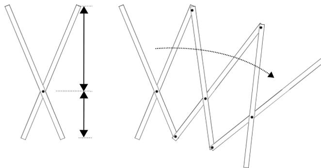
**Figure 3.37:** Straight elements attached with eccentricity yield polar structure
