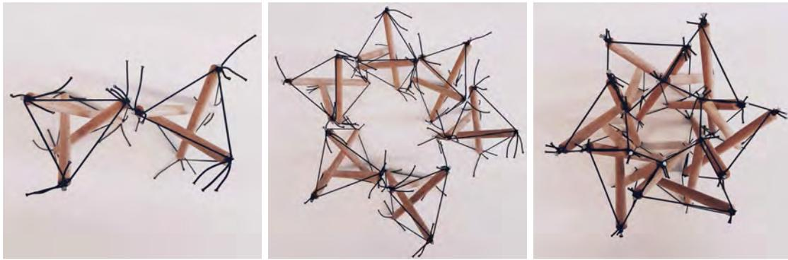
**Figure 4.28:** Triangular tensegrity modules to be assembled to triaxial weave
