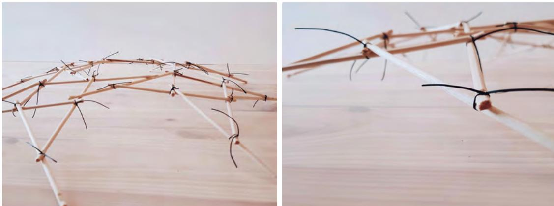
**Figure 5.13:** Physical model of four reciprocal lace bindings
