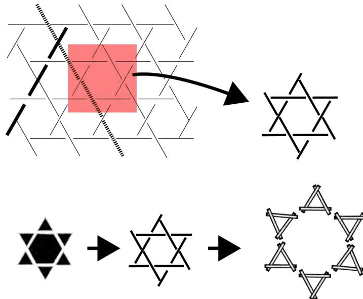
**Figure 4.23:** Triaxial weave analysis, identified joint mapped to a structure
