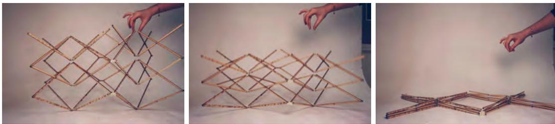
**Figure 4.4:** Without friction in the joints the structure is a mechanism (image from ArcInTex workshop at NTU, held by Marisela Mendoza)
