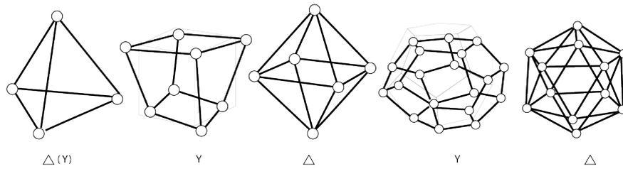
**Figure 3.18:** Platonic lattice structures; stable -  $\Delta$ , movable -  $Y$ . Redrawn from *Structural order in space* by T.Wester [19]
