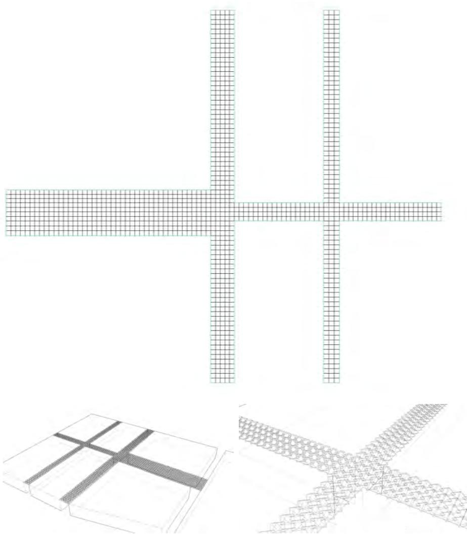
**Figure 6.3:** Grid adapted to the geometry of the roof surface in which the scissor structure can be placed (top) and scissor structure positioned along this grid
