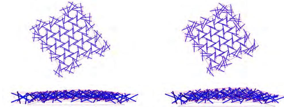
**Figure 6.21:** Influence of cable length during Kangaroo form finding - same length top and bottom (left), shorter length bottom (right)
