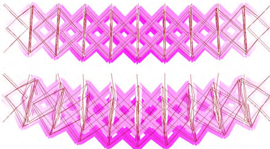
**Figure 6.11:** Deflection of platonic scissor structure with rigid (upper) and semi-rigid (lower) connections, maximum deflection: 39mm and 128mm respectively
