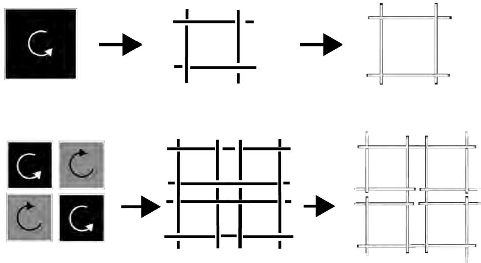
**Figure 4.20:** Plain and double weave joints mapped to their respective reciprocal structures
