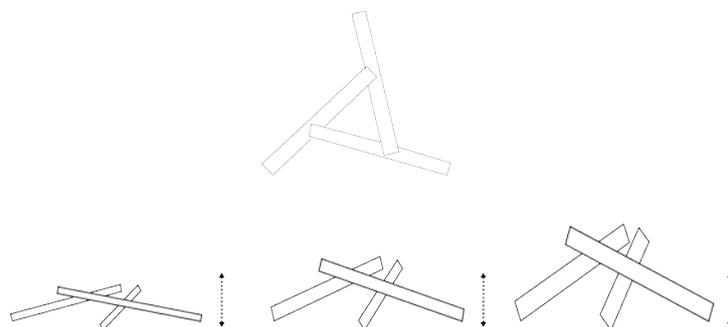
**Figure 3.34:** Relationship between height of elements and the global height in a reciprocal structure
