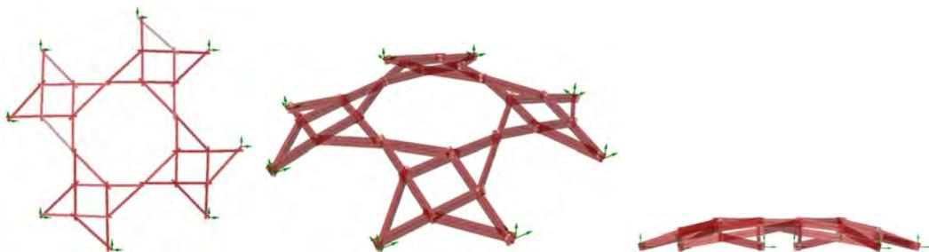
**Figure 6.28:** Undeformed digital model of reciprocal lace structure from Karamba analysis
