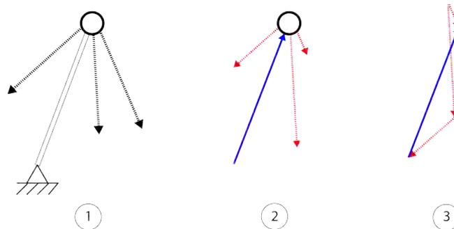
**Figure 3.26:** Equilibrium attained in a tensegrity structure by attaching one node on the lattice with three tensile bands
