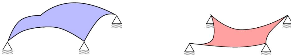
**Figure 3.24:** Surface-active structural systems
