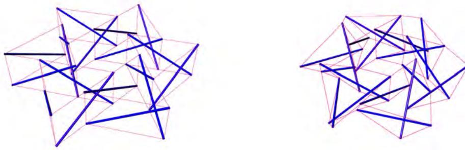
**Figure 5.11:** Form finding of a tensegrity weave module with shorter tension bands on the bottom side
