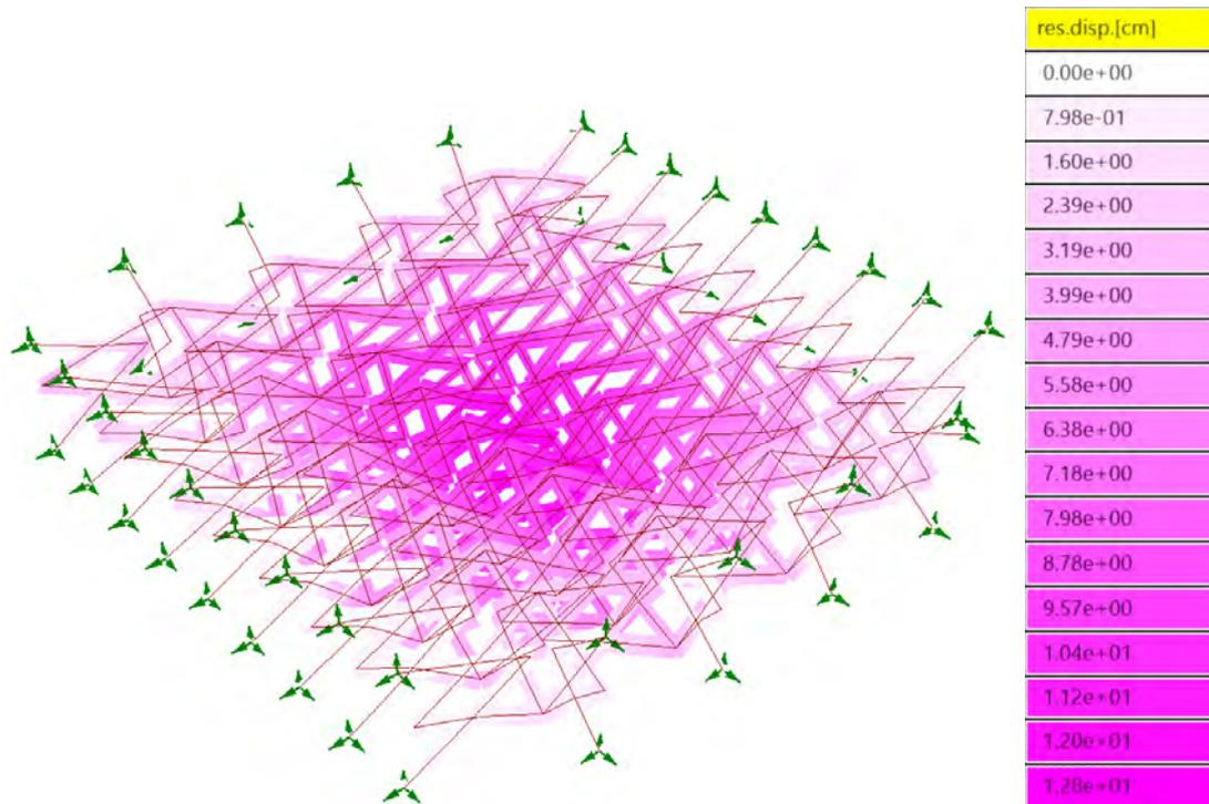
**Figure 6.10:** Deformed digital model of the platonic scissor structure, with semi-rigid connections, maximum deflection: 128mm
