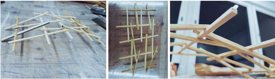
**Figure 2.5:** The da Vinci bridge - a reciprocal model of a weave
