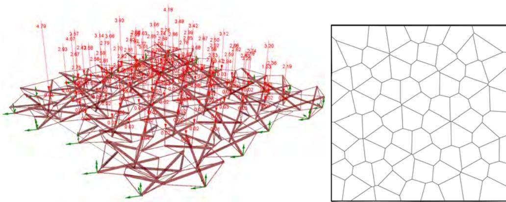
**Figure 6.23:** Loads applied to the digital model (left) - from textile roof cover and snow load - and its distribution (right)
