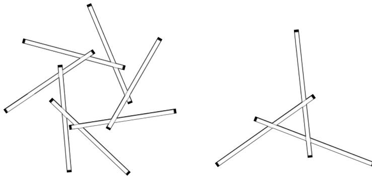
**Figure 3.32:** Figure of two reciprocal structures of three and seven pieces
