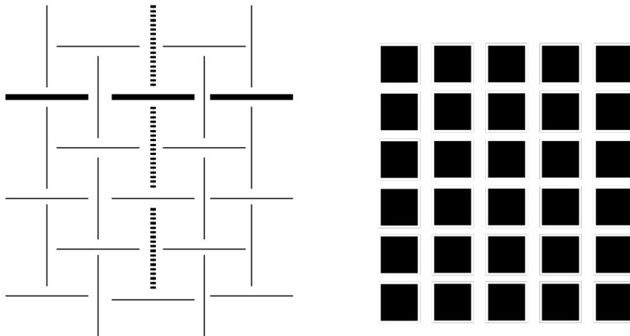
**Figure 4.14:** The geometric interpretation of a plain weave - 2D array of squares
