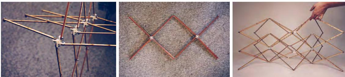
**Figure 4.3:** Three-dimensional joints make it possible to assemble octahedron scissor structures next to each other (image from ArcInTex workshop at NTU, held by Marisela Mendoza)
