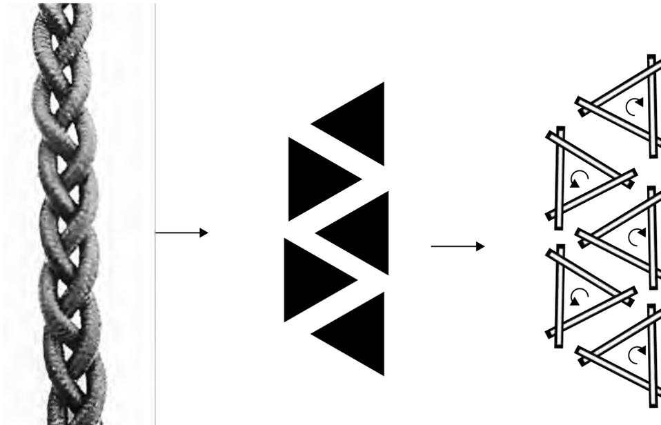
**Figure 4.11:** Geometric pattern of a braid interpreted to a combination of reciprocal structures
