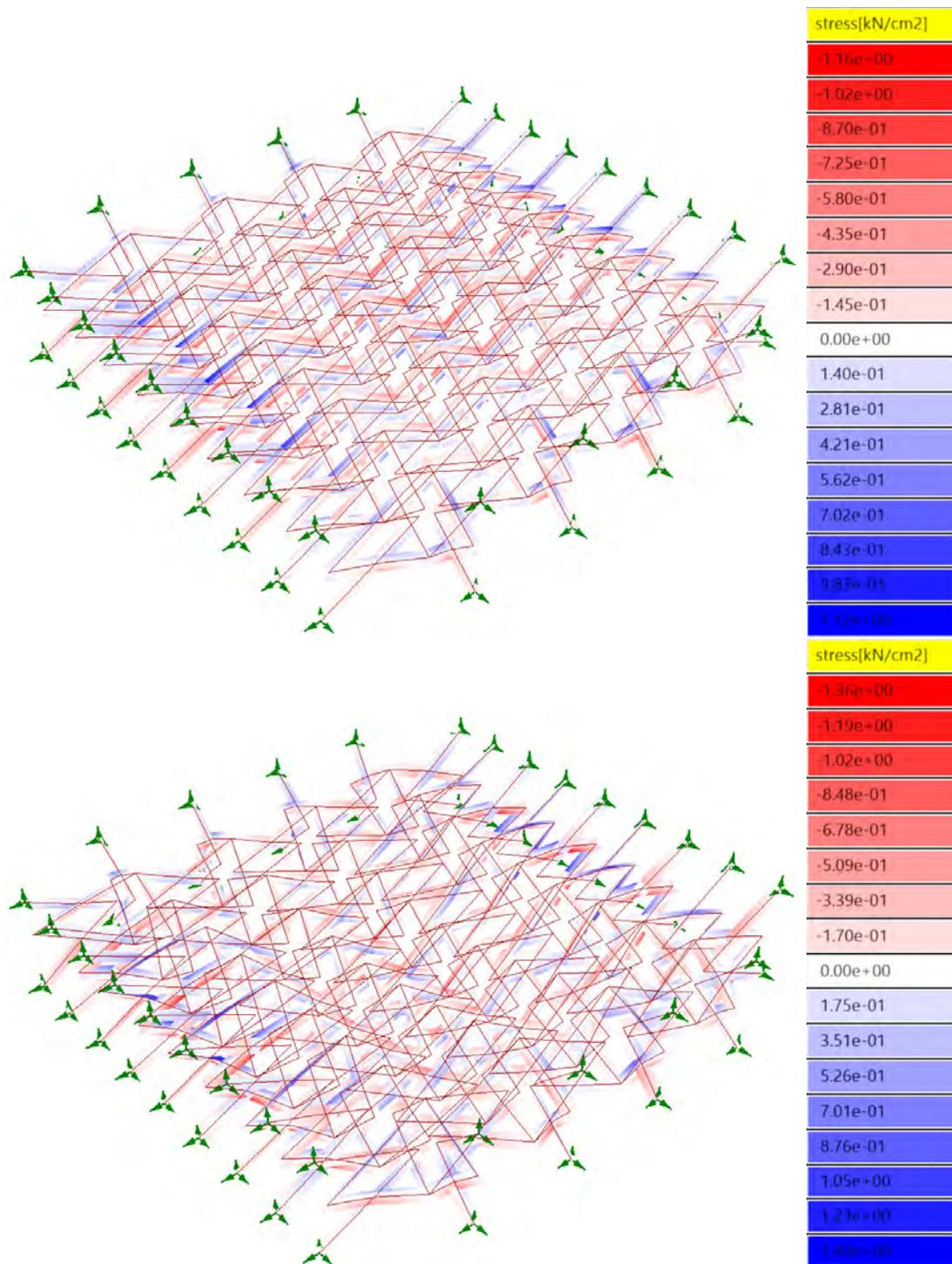
**Figure 6.12:** Axial stress distribution of platonic scissor structure with rigid (upper) and semirigid (lower) connections
