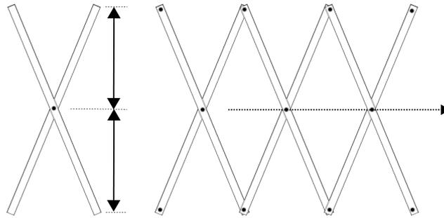
**Figure 3.36:** Straight elements attached at the middle yield a transverse motion
