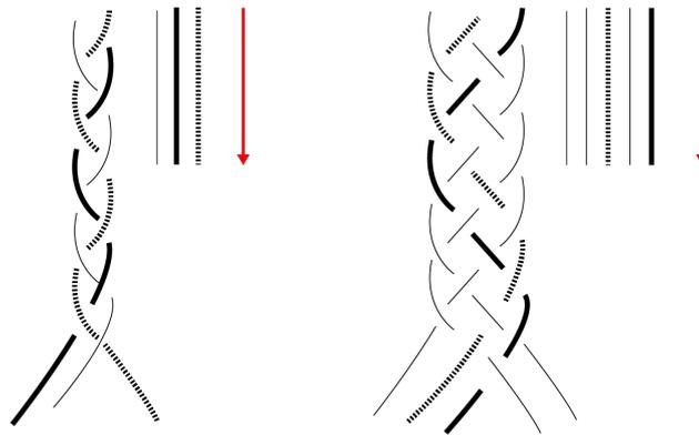
**Figure 3.2:** Braid of three and braid of five, red arrow indicating braid direction
