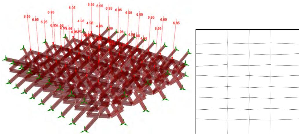
**Figure 6.9:** Loads applied to the digital model (left) - from textile roof cover and snow load - and its distribution (right)
