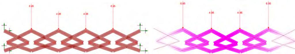
**Figure 6.17:** *Asymmetric* modules in a straight line with two supports on each side and a module length of 3.75 m and height of 1.4 m, *rigid* connections throughout. Undeformed (left) and deformed (right)
