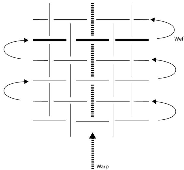
**Figure 3.7:** Warp and weft direction in a plain weave
