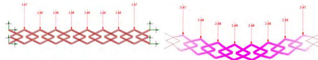
**Figure 6.18:** Symmetric modules in a straight line with two supports on each side and a *module size of 1.85x0.94 m*, *rigid* connections throughout. Undeformed (left) and deformed (right)
