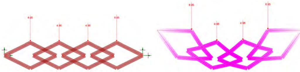
**Figure 6.16:** Symmetric modules in a straight line with *one* support on each side and a module size of 3.75x1.88, *semi rigid* connections throughout. Undeformed (left) and deformed (right)
