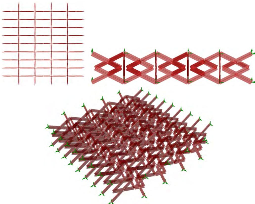
**Figure 6.8:** Input geometry for Karamba analysis of platonic scissor structure
