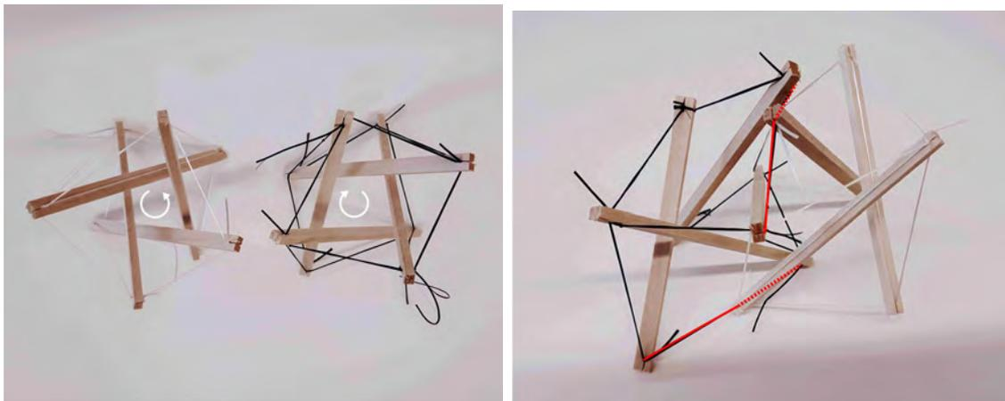
**Figure 4.27:** Assembly of two reverse turned tensegrity modules - one module is attached to the middle of the tension bands on the neighbouring module
