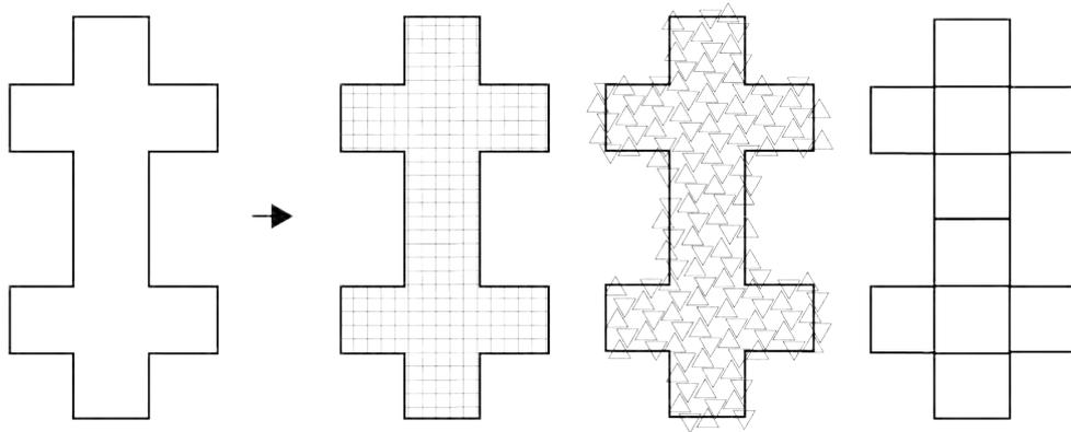
**Figure 6.2:** Geometrical application of the three different concept on the roof geometry: scissor structure is placed according to a grid; tensegrity modules are placed according to a pattern where modules outside of the surface are excluded; reciprocal lace, division of the surface is made into a few smaller squares where an edge beam is assumed.
