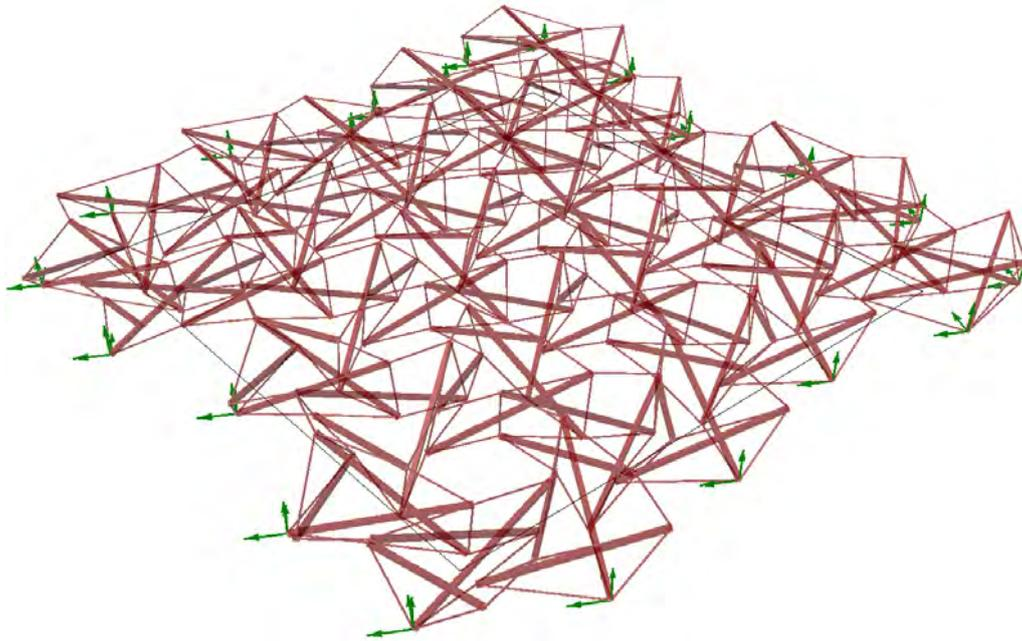
**Figure 6.24:** Undeformed digital model of tensegrity weave structure from Karamba analysis
