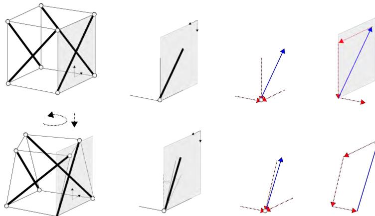
**Figure 3.28:** Figure and force diagram of a tensegrity module before and after form-finding to a null stress equilibrium geometry
