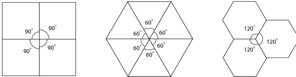
**Figure 3.15:** Regular polygons where the corner angle is a sub-multiple of 360 can cover a flat surface continuously
