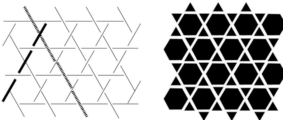
**Figure 4.16:** Geometric interpretation of a triaxial weave yields a pattern of hexagons and triangles
