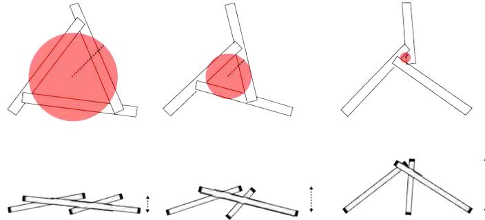
**Figure 3.33:** Relationship between height and inner radius in a reciprocal structure, top view and corresponding side view
