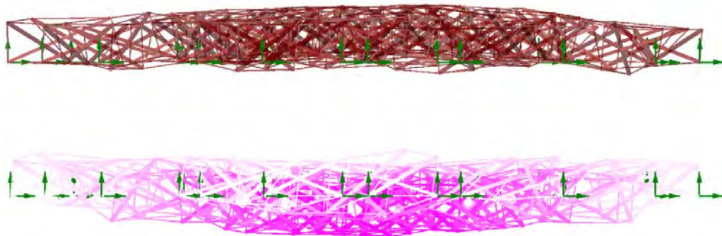
**Figure 6.25:** Undeformed (upper) and deformed model (lower) of tensegrity weave structure from Karamba analysis
