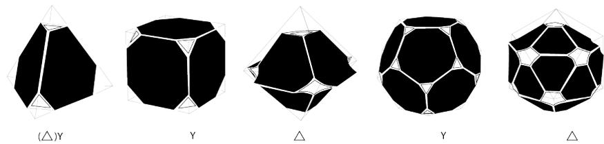
**Figure 3.19:** Platonic plate structures; stable -  $Y$ , movable -  $\Delta$ . Redrawn from *Structural order in space* by T.Wester [19]
