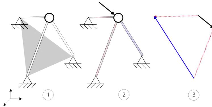
**Figure 3.25:** Equilibrium state of a stable point in three dimensions, under a load
