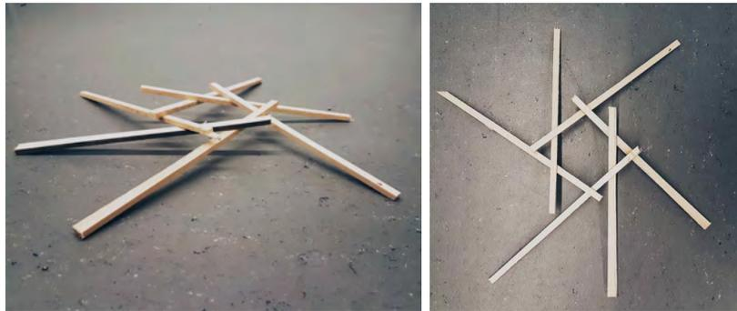
**Figure 3.31:** Reciprocal model of a hexagon
