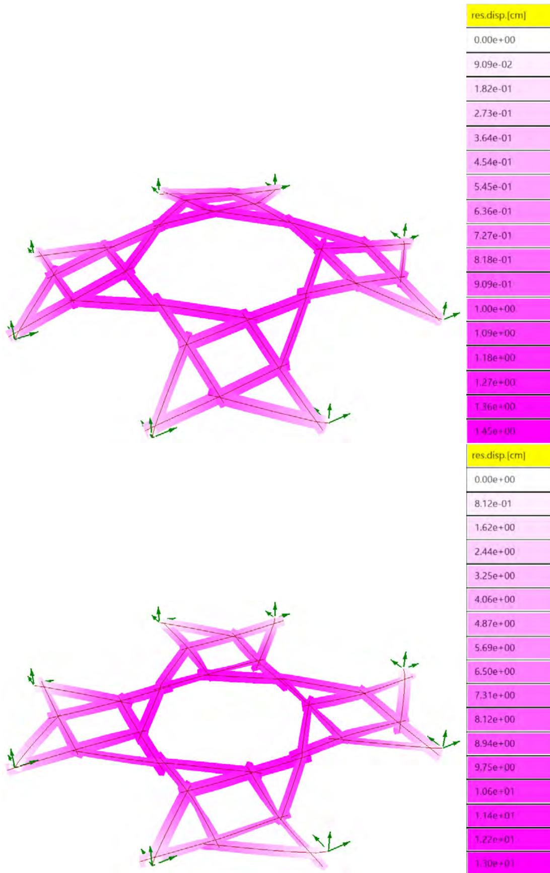
**Figure 6.30:** Deformed model of reciprocal lace structure from Karamba analysis, rigid connections (left) and semi-rigid connections (right)
