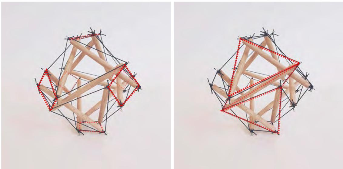
**Figure 4.7:** All sides are triangulated with tension bands, except for truncations which stay as squares
