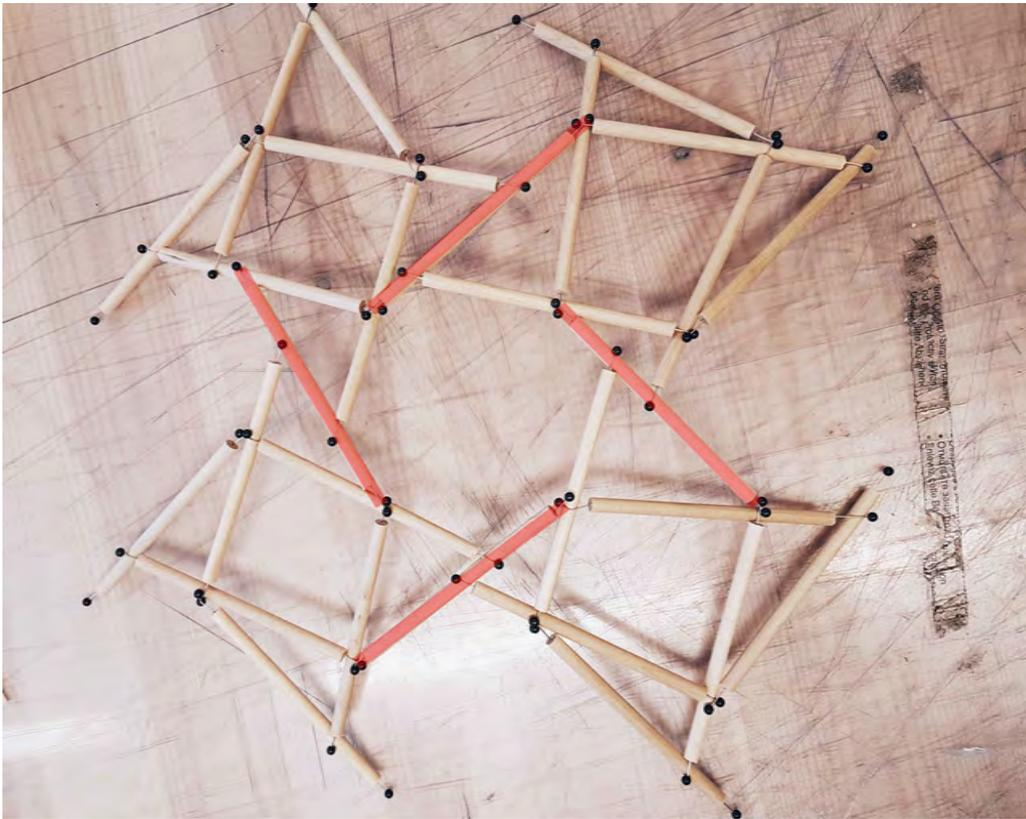
**Figure 4.35:** Reciprocal model of a bobbin lace with diagonal elements replacing the twisted yarns
