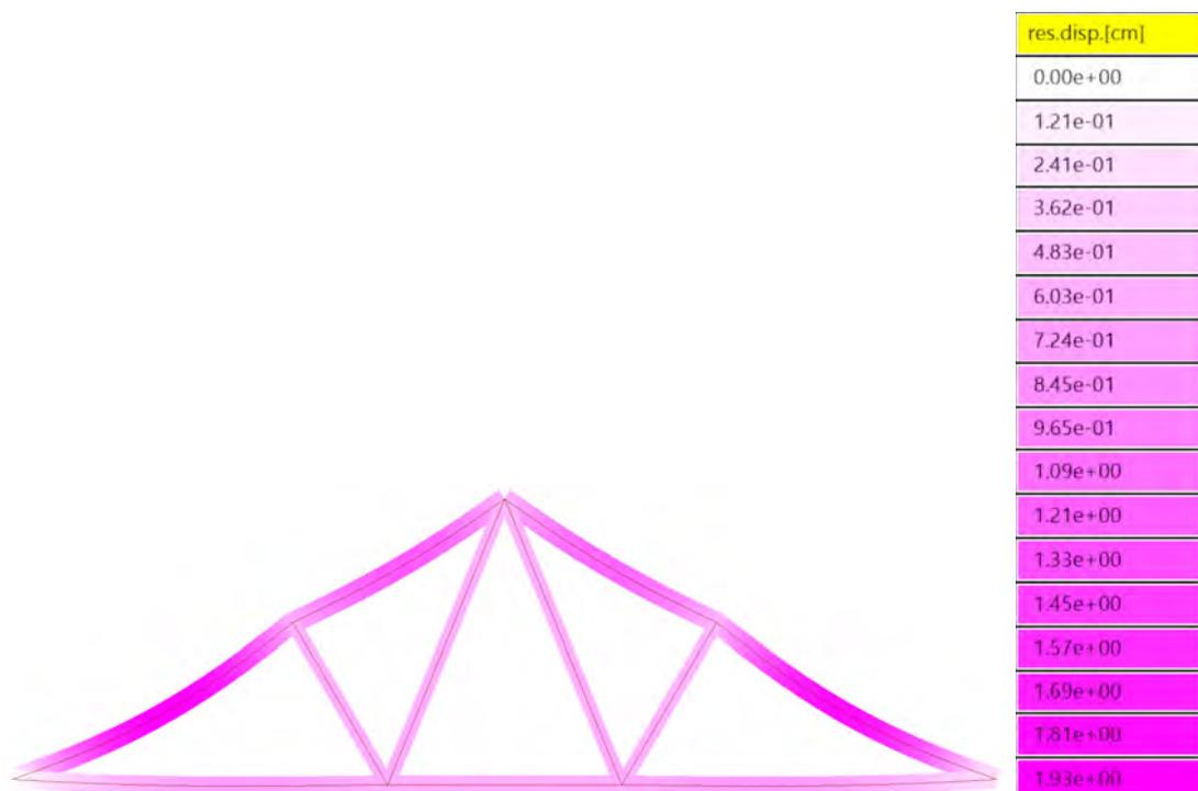
**Figure 6.6:** Displacement of roof truss analysed with Karamba, the deformation is scaled x10 in the figure
