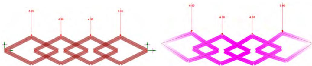
**Figure 6.15:** Symmetric modules in a straight line with *one* support on each side and a module size of 3.75x1.88 m, *rigid* connections throughout. Undeformed (left) and deformed (right)
