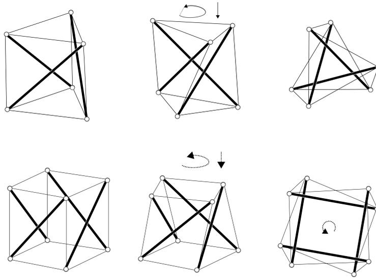
**Figure 3.27:** Form-finding of a tensegrity modules of three and four rods
