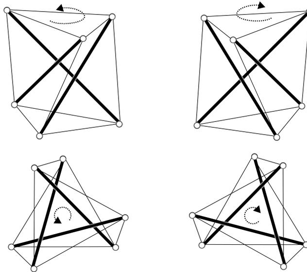
**Figure 3.29:** Tensegrity modules of three rods, one left turned and one right turned
