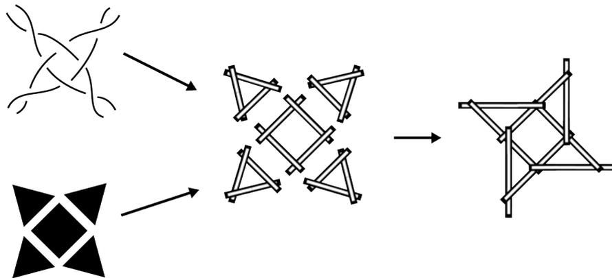
**Figure 4.34:** Joint translated to structure in reciprocal lace
