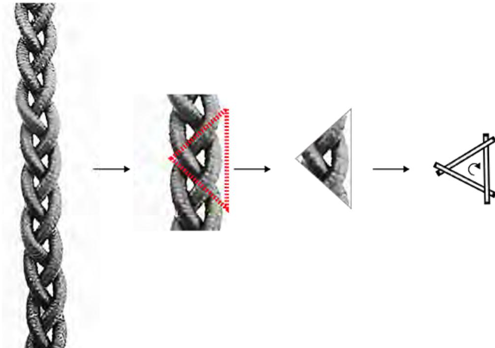
**Figure 4.10:** Interpretation of a triangular section of a braid
