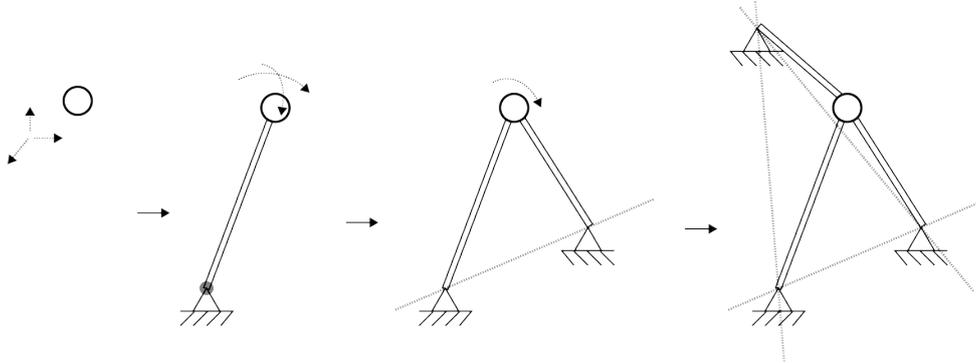
**Figure 3.17:** A stable point in space must be connected by three non co-planar rods
