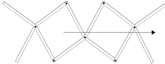
**Figure 3.40:** Angled scissor modules attached to a polar structures
