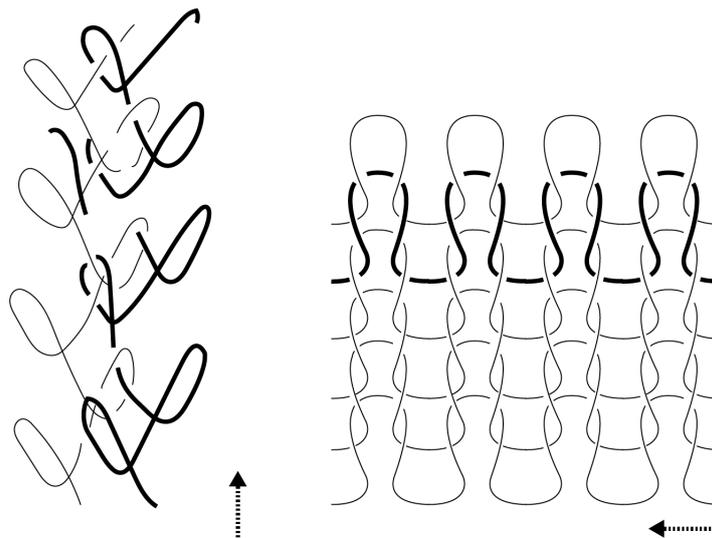
**Figure 3.14:** Figure of knit methods, left; warp knit, right; weft knit
