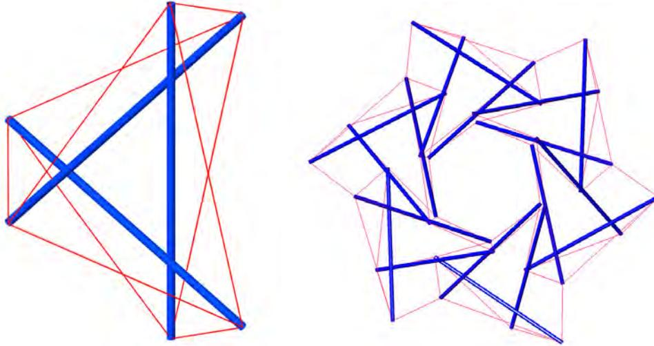
**Figure 5.8:** Digital tensegrity module into a tensegrity triaxial weave binding module
