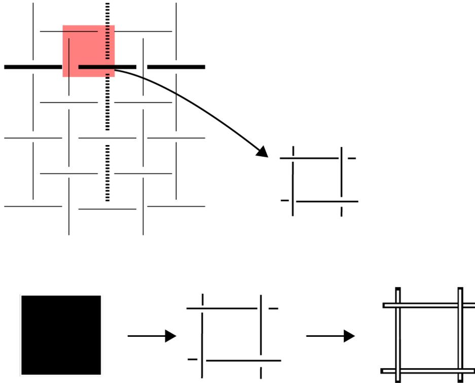
**Figure 4.17:** Plain weave analysis, joint resemblance to a reciprocal module
