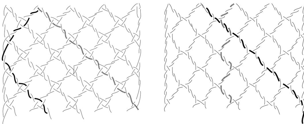
**Figure 3.6:** A Hole Ground lace (left) and a Tulle Ground lace (right) with two thread paths marked
