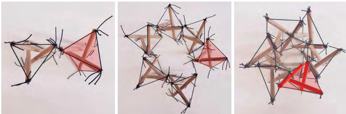
**Figure 4.29:** Triangular tensegrity modules to be assembled to one triaxial weave tensegrity module
