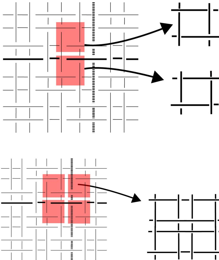
Figure 4.19: Plain versus double weave analysis, joint mapped to a structure
