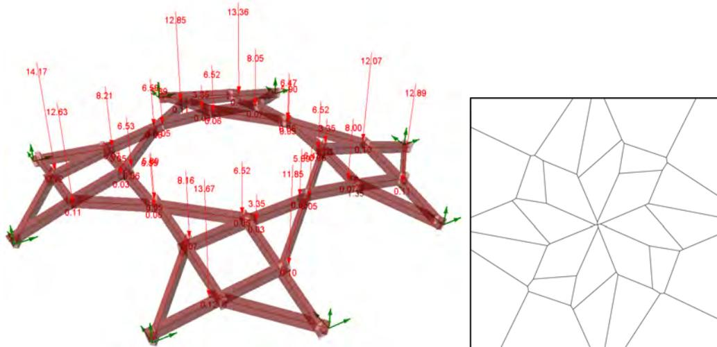
**Figure 6.29:** Loads applied to the digital model (left) - from textile roof cover and snow load - and its distribution (right)
