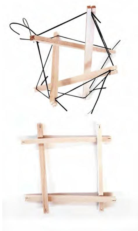
**Figure 4.1:** When realising the tensile bands of the tensegrity module (top) and thus relaxing the structure, a reciprocal frame is obtained (bottom)
