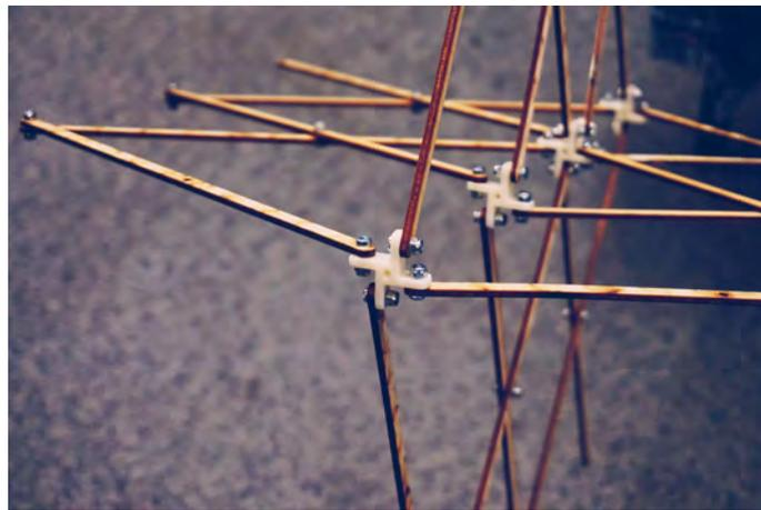
**Figure 3.41:** Three-dimensional joints for scissor structures (image from ArcInTex workshop at NTU, held by Marisela Mendoza)
