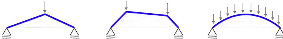
**Figure 3.21:** Form-active structural systems working in pure compression
