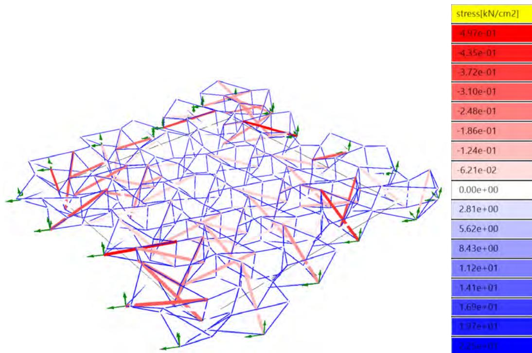
**Figure 6.27:** Axial stress distribution of tensegrity weave structure, analysed with Karamba. Compression in red, tension in blue.
