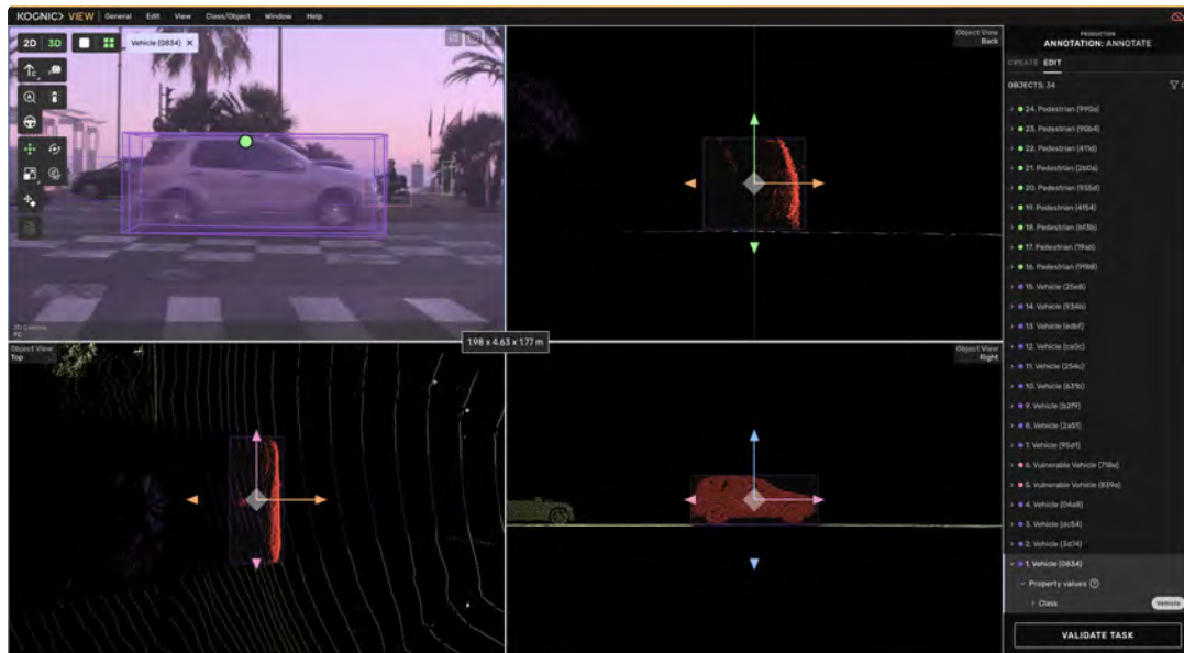
Figure 7.7: Grid View mode while annotating in the Kognic Platform. Used while fine-tuning the cuboid. Screenshot provided with consent from Kognic.
