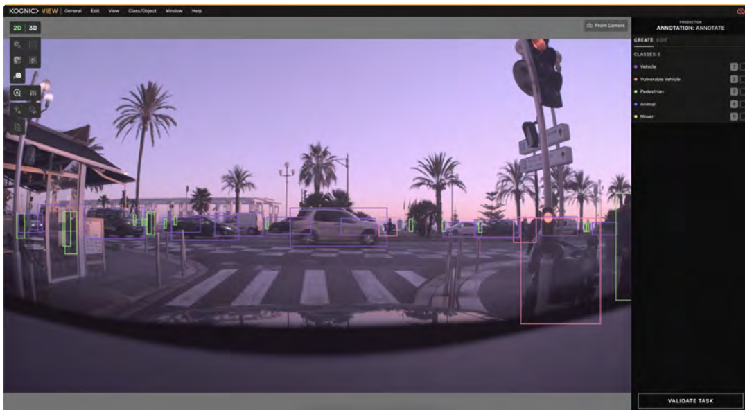
Figure 7.4: 2D view mode while annotating in the Kognic Platform. Vehicles have been marked out using boxes. Screenshot provided with consent from Kognic.
