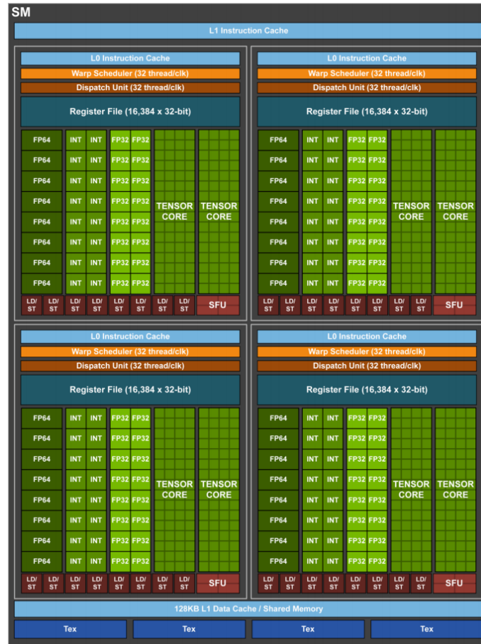
Figure 2.1: The Nvidia Volta streaming multiprocessor (SM). Most required hardware for computation resides within the SM. Note that each marked computational unit in the figure, e.g. the marked FP64 units, is here a streaming processor and consists of 32 ALUs in total. Also noteworthy is the tensor cores which takes up nearly half of the space for computational units and by its restricted execution of half-precision 4 \times 4 matrix FMA (Fused Multiply Add) operations cannot be readily utilized for many applications. [16]
