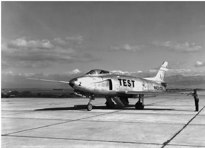
Figure 1.1: North American YF93A used by NACA as a test platform for submerged inlets
