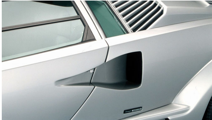
Figure 1.2: NACA duct on a high performance car
