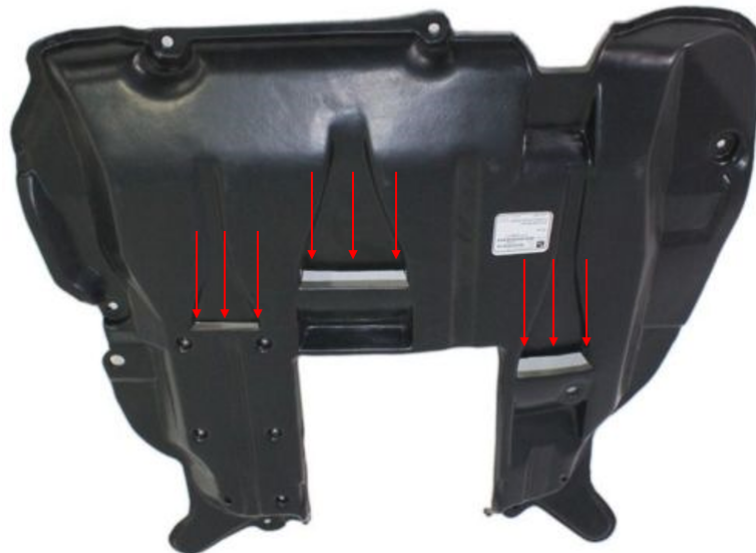
Figure 1.3: Engine under shield with integrated NACA ducts
