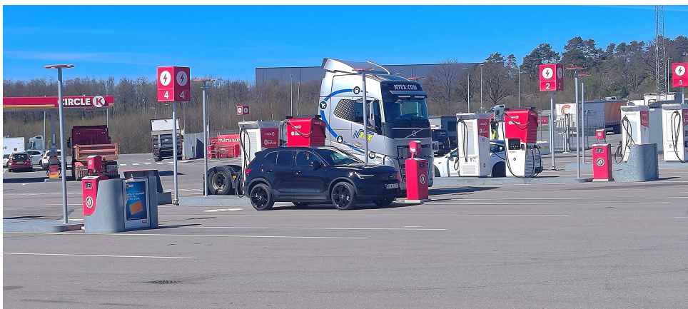
Figure 4: Shows two electric cars and one electric truck charging using chargers intended for trucks.
