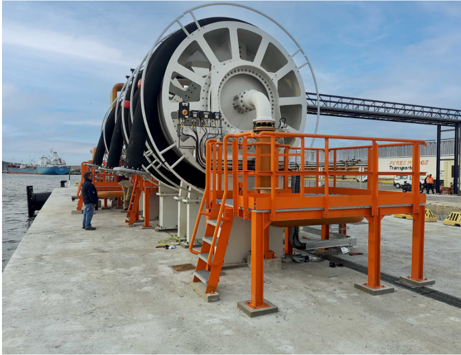
Figure 2.2: A DockReel marine loading hose installation in use. Image sourced from [42].
