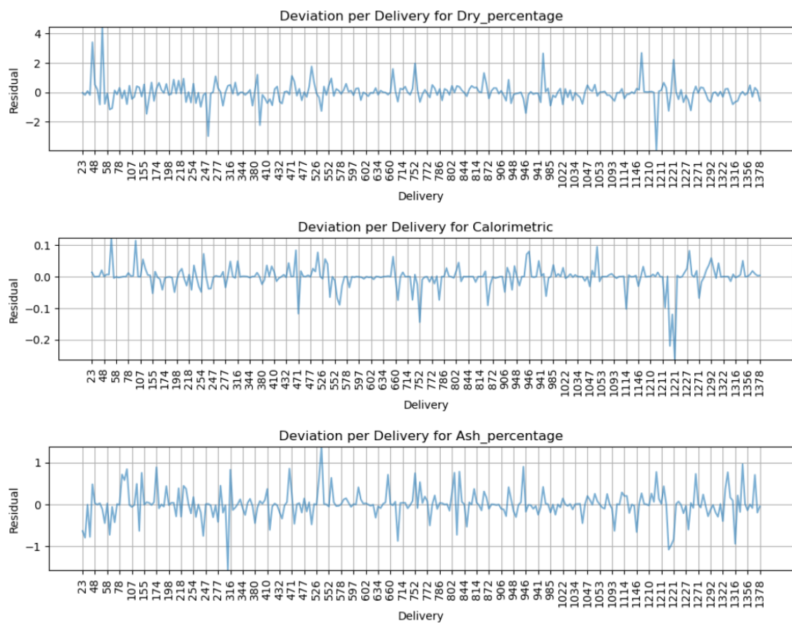
Figure A.11: Plots displaying residuals for each parameter using XGB.
