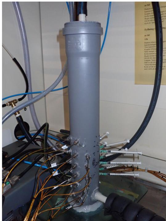
**Figure 3.4:** The small fabricated canister.
