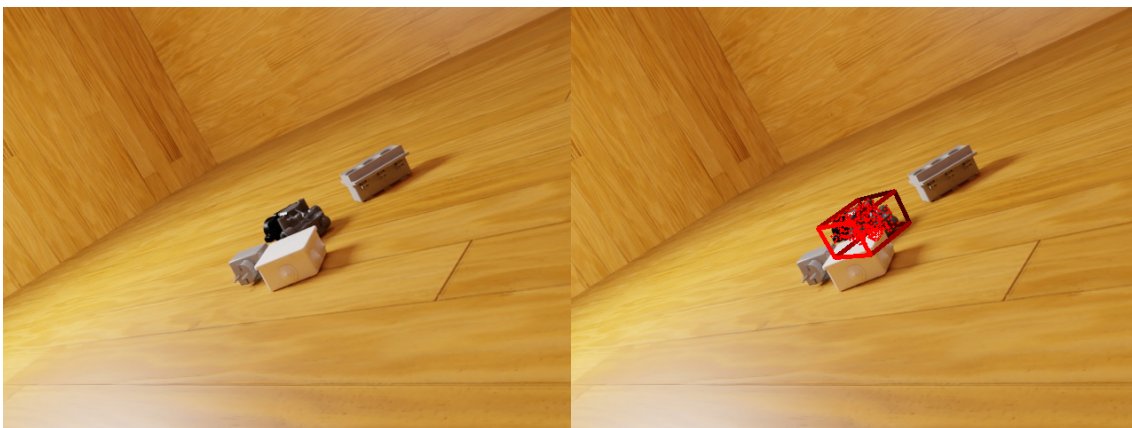
Figure 4.19: Point cloud and 3D bounding box in overlapped data
