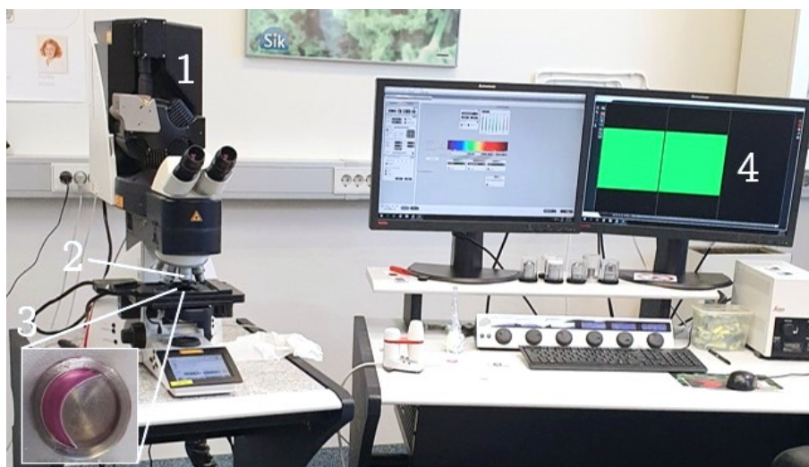
Figure 3.2: CLSM instrument. (1) is the microscope, (2) is the objective, (3) shows the sample setup and (4) is the monitoring screen.
