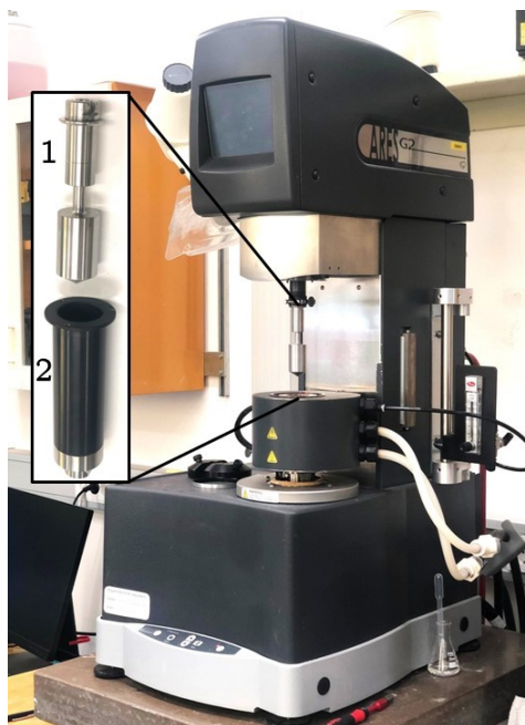
Figure 3.4: Rotational rheometer. (1) is the bob and (2) is the cup.
