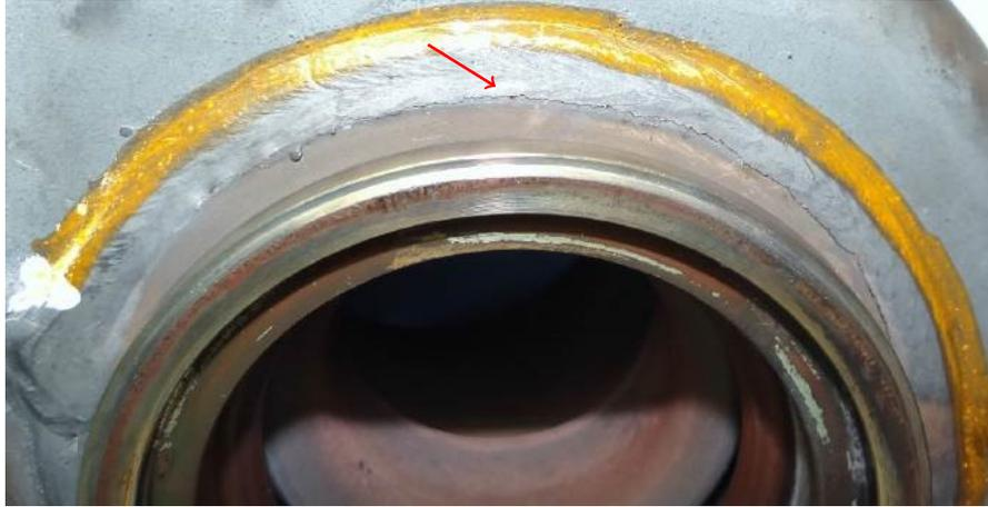
Figure 3.2: *Weld toe crack in a test engine after a thermal shock test.*
