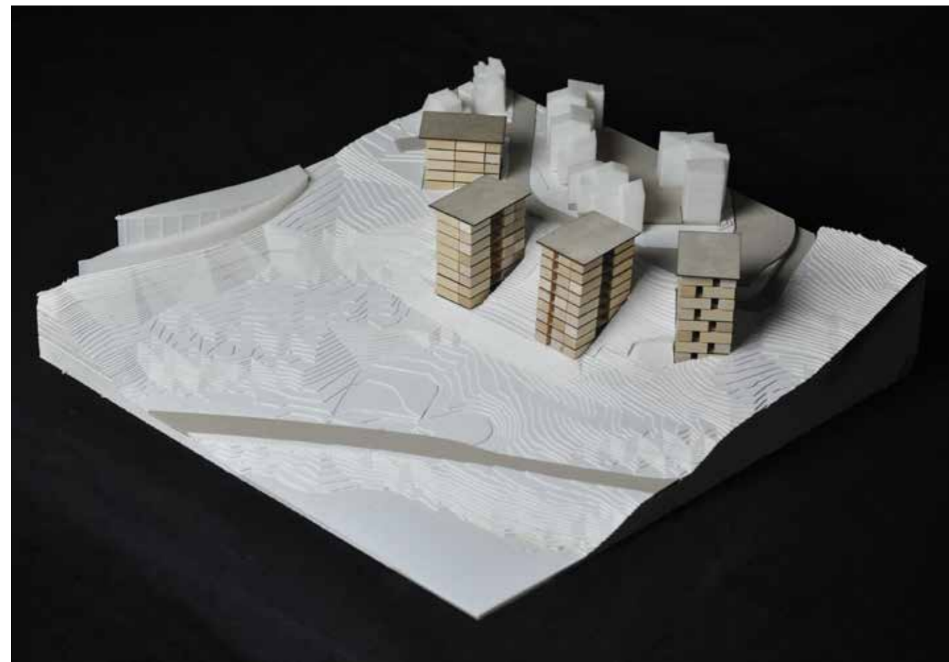
Model photo Volume Elements reinterpret in light frame and CLT. The structures with overlapping volume elements are reinterpreted as they were made
