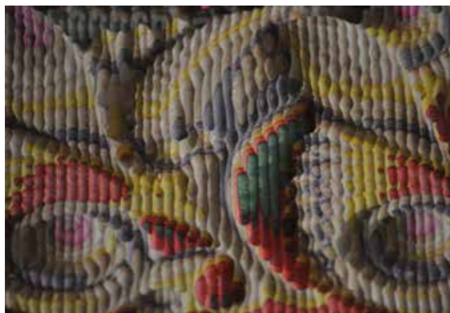
A 8 mm drill bit was used in this test. The surface was left fairly rough for its ornamental purposes.
