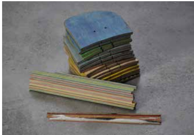
Model Photos: Reused material such as used up skateboards could be reused in a wooden gluing and milling process.
