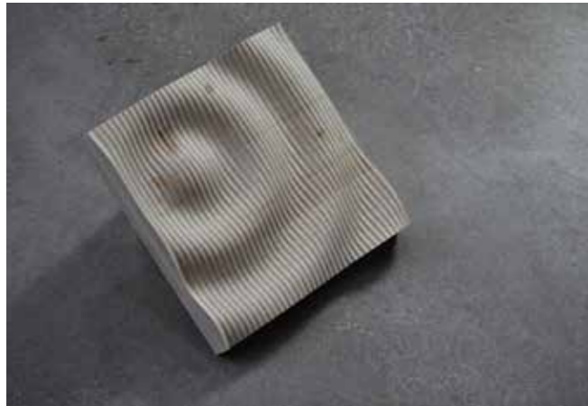
Milled piece CLT 1:2 350x350x65 Milling time: 10 min
