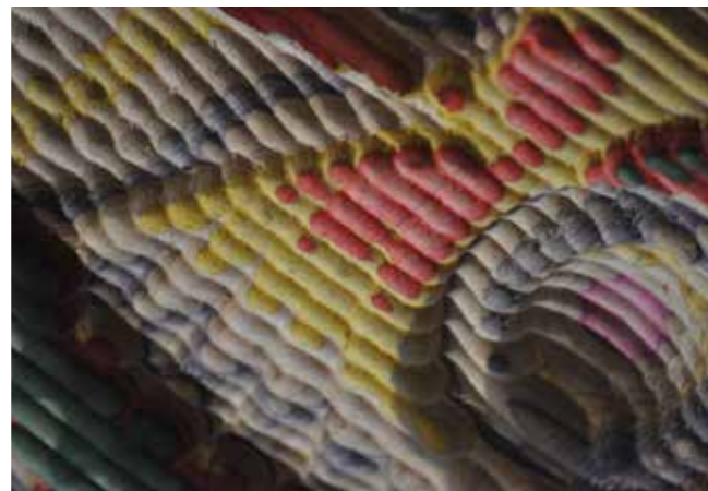
Close-up of the rich colours of the glued and milled veneers.
