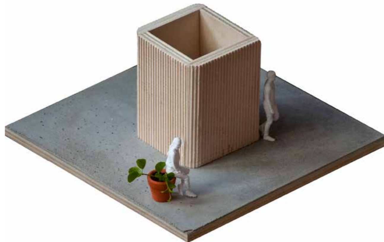
Model study in 1:20 scale, testing how to mill round corners with a striped pattern on a CLT-core
