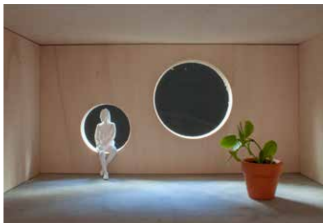
Model Photos Row 3: Perforations are not restricted to be shaped in an orthogonal way when made with a CNC-mill. The round shape of the milling
