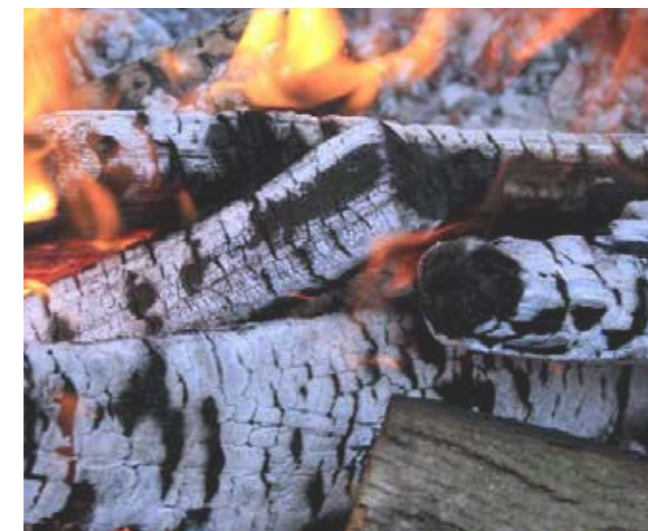
Figure 6. The charred parts of wood have low thermal conductivity which slows down the fire process, after 60 minutes of fire the char have penetrated approximately 40 mm into a wooden beam. (Pixnio, n.a.)
