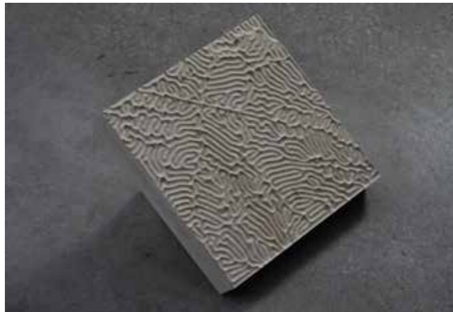
Milled piece CLT 1:2 350x350x65 Milling time: 5 min
