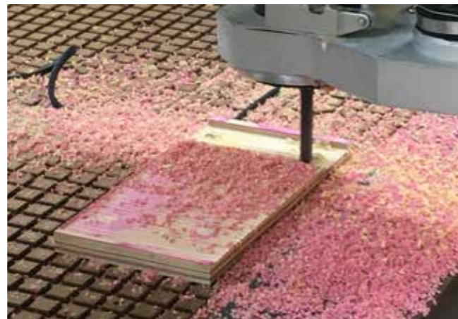
A 3 axis mill together with computing software was used to re-create a scanned geometry of an already existing ornament.
